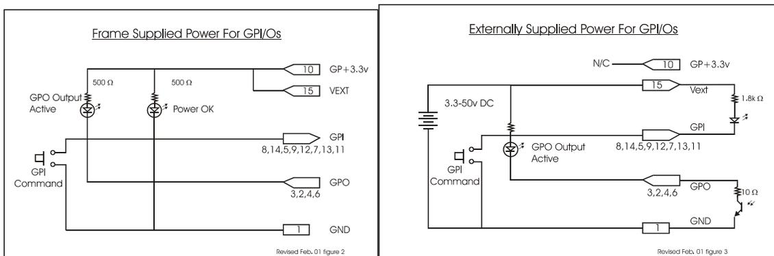
Alternately, an external voltage source may be applied (see figure 3). The Vext voltage must be greater than the voltage supplied to GPI by at least 3v.
