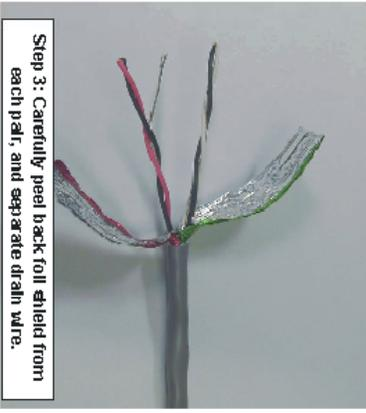
Step 3: Carefully peel back foil shield from each pair, and separate drain wire.
