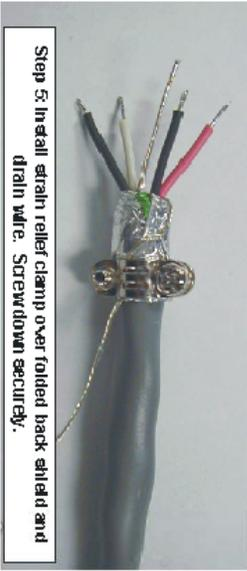
Step 5: Install drain roller clamp over folded back shield and drain wire. Screwdown securely.
