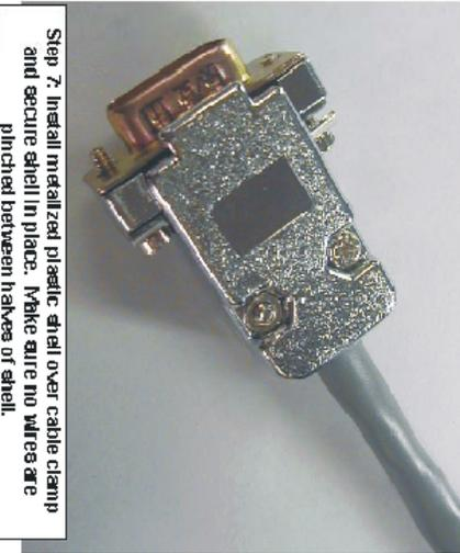
Step 7: Install metallized plastic shell over cable clamp and secure shell in place. Make sure no wires are pinched between halves of shell.
