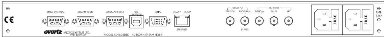
Connect the incoming video to the *HD Input BGNDA*, input BNC connector for HD serial digital SMPTE 292M video. A video signal should be supplied prior to applying power to the box.
