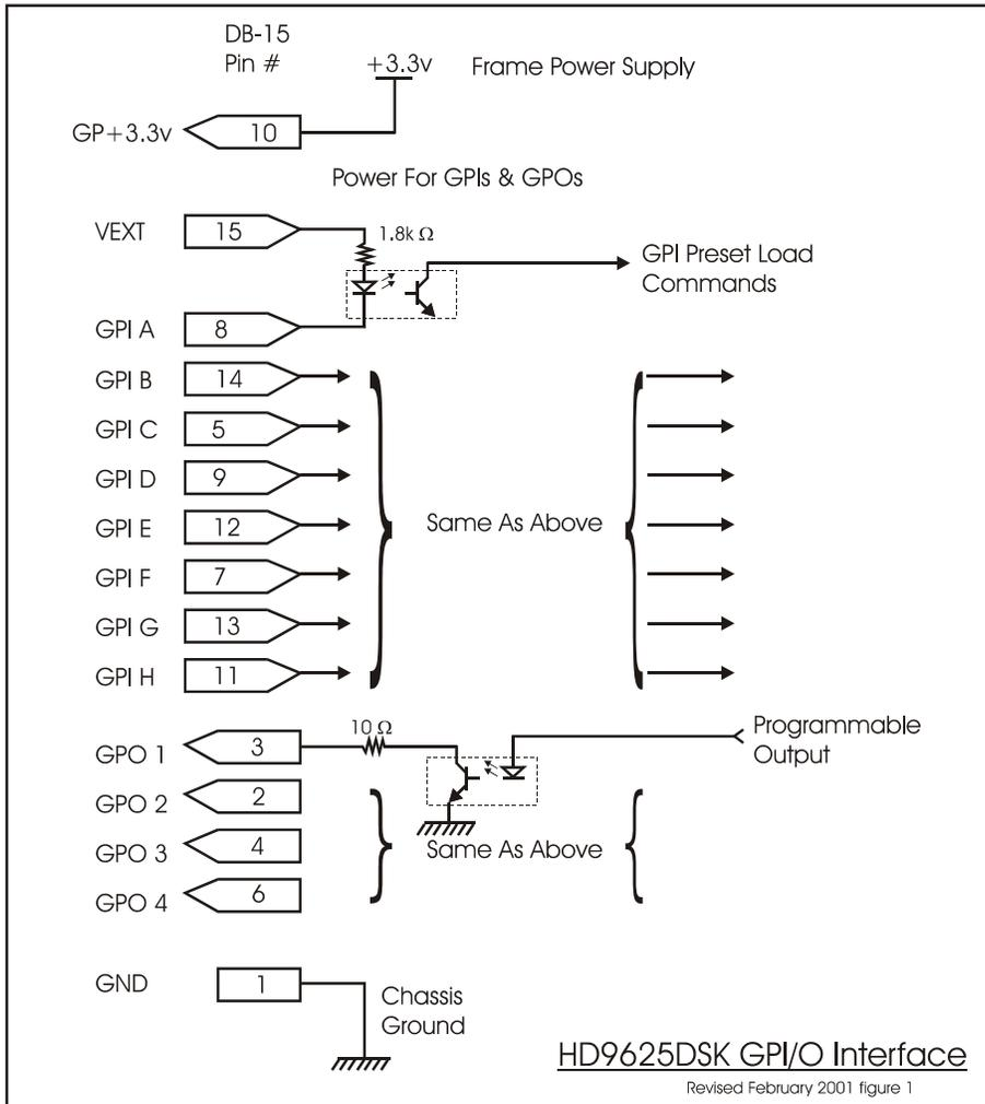
All GPI inputs are level triggered. Lowering the GPI input to a potential below Vext will select the allocated preset definition. The 8 GPIs (A through H) are dedicated as preset load controls. When one of these GPI inputs are activated, the corresponding preset configuration is loaded. If multiple inputs are active both commands are ignored until a single input is recognized.
