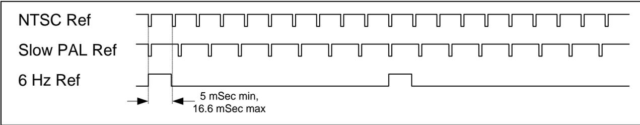
**Figure 4-1: 6 Hz Reference Pulse Timing**
