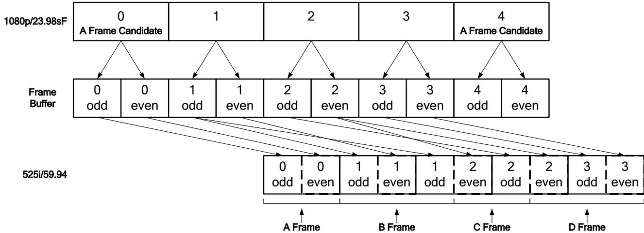
Figure 3-5: 2:3:3:2 Pulldown Sequence – 23.98 Fps Input Video
