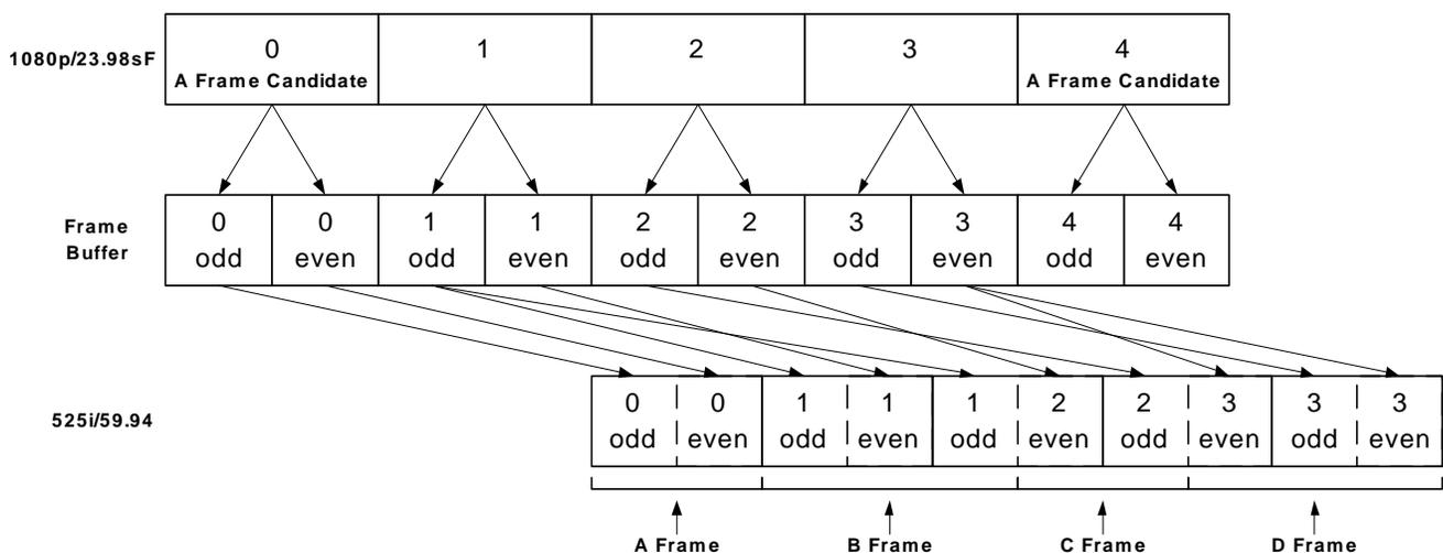
Figure 3-4: 2:3:2:3 Pulldown Sequence – 23.98 Fps Input Video
