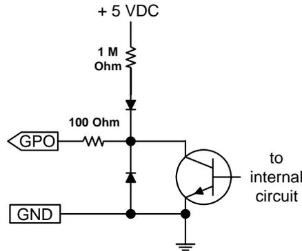
Figure 2-8: General Purpose Output Schematic
