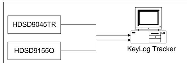
**Figure 2-10: Connecting KeyLog TRACKER™ to HDSD9045TR and HDSD9155Q using 2 COM Ports**
