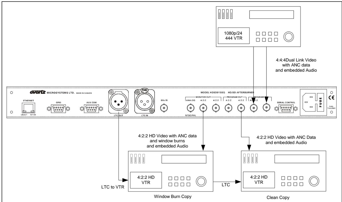
**Figure 2-5: HD In – HD Out Typical Configuration**
