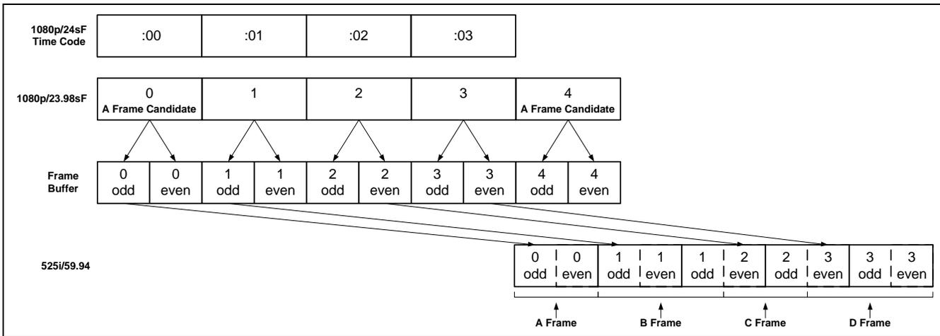
Figure 4-3: Timecode Referenced 2:3 Pulldown and Delay
