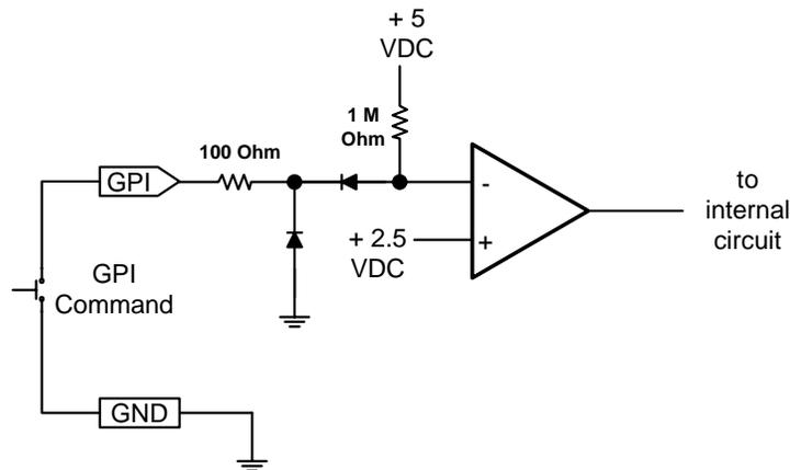
Figure 2-7: General Purpose Input Schematic
