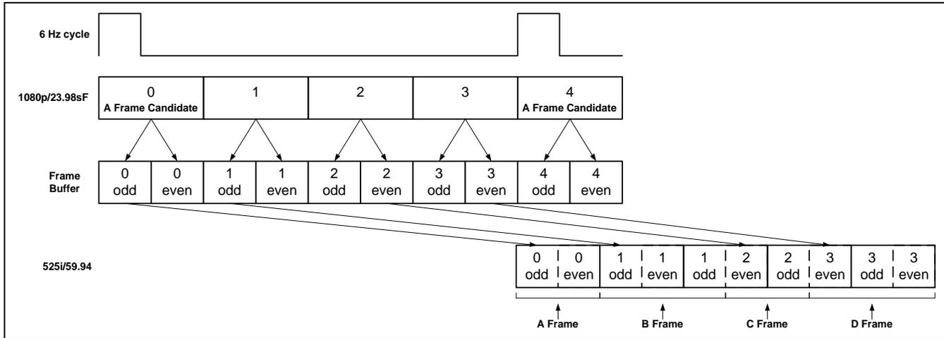
Figure 4-2: 6 Hz Referenced 2:3 Pulldown and Delay
