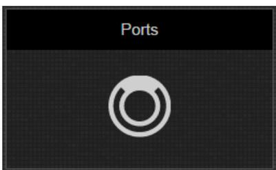
This opens the **Ports** application directly from the dashboard. The **Ports** app provides the user with the ability to name the source and destination ports within the system. It additionally provides engineering level routing through the system.
