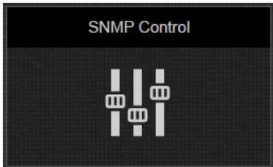
This opens the **SNMP Control** application directly from the dashboard. The **SNMP Control** app provides the user with the ability to create configurations or status views for the hardware that MAGNUM is interfacing to.
