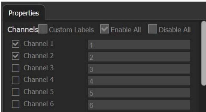
This *Properties* tab is associated with the Level Bar widget. It allows the user configure the number of audio channels the selected Level Bar widget will display and the mapping of those channels.
