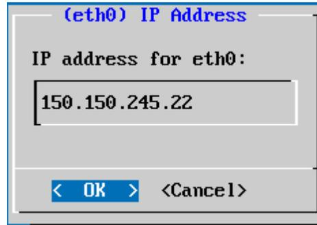
Figure 3-13: Enter IP Address for eth0
