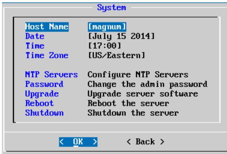
Figure 3-2: System Configuration Menu
