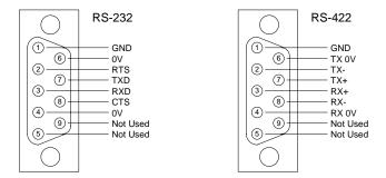
The cable between the PC and the router (RS232) only needs to use TX, RX, and GND as shown below.
