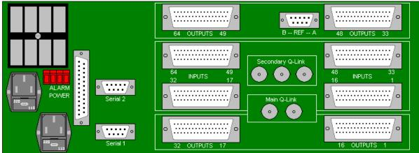
For digital audio it is important to use data cable with a characteristic impedance of  $110\Omega$  rather than audio cable. For error free transmission, care should be taken to ensure the cable losses are acceptable over the intended length.
