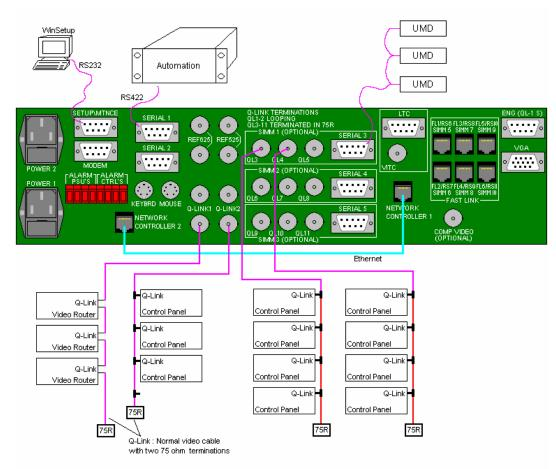
As a system design guide the SC-1000 should be considered when the router grows above 128x128 single level or has more than 10-15 total Q-Link devices. See section 6.10 for further information on the SC-1000.
