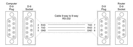
The computer port connector on the rear of a remote control panel only functions if a CI-0003 module is installed. Controlling the routing system through a panel computer port is possible but is not recommended, these ports are only provided for stand-alone S7 panels i.e. CP-3200-S7.
