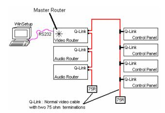
To allow re-configuration, all systems are supplied with WinSetup, which is a Windows program enabling the user to edit the PC based setup files and then download the selected file to the router.
