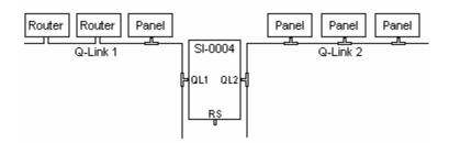
In large buildings the SI-0004 would only be installed once a problem had been identified. In OB trucks it is good practice to install an SI-0004 between the internal Q-Link and any external 'tail gate' or bulk head patch panels. Multiple SI-0004 units can be used where several external Q-Links are required.
