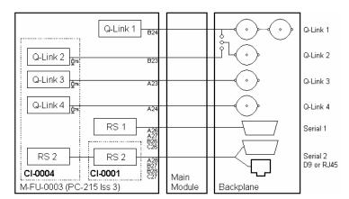
For real time or high-speed control it is essential that the serial port on the master router be used. As Serial 1 is normally required to configure the routing system from WinSetup, Serial 2 would normally be used for the high-speed connection and this requires a CI-0001 or CI-0004 module.
