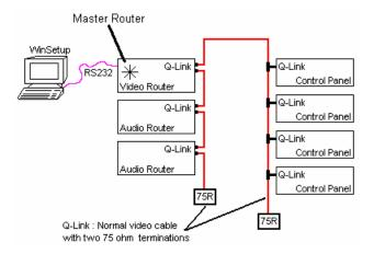
This daisy chain method ensures the best transmission quality of the control signals down the cable. Short cuts that might save cable, such as running stubs to some panels, are not recommended as this may cause data errors under certain circumstances. The maximum cable length is shown in the Technical Specification in Section 2 of this manual.
