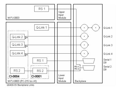
All Quartz products use the same pin-out for the serial D9 connectors. The wiring of the connectors is different for RS232 and RS422.
