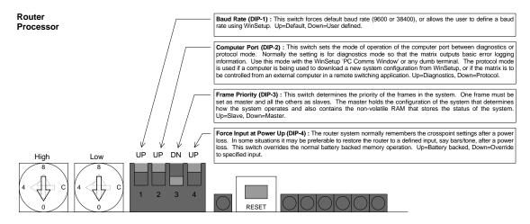
The reset switch must be pressed after changing the DIP switch.
