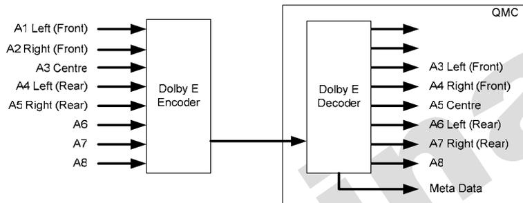
The Meta data that is extracted from the Dolby E signal during the decoding process is passed onto the RJ 45 connector where it becomes available as a serial RS422 signal.
