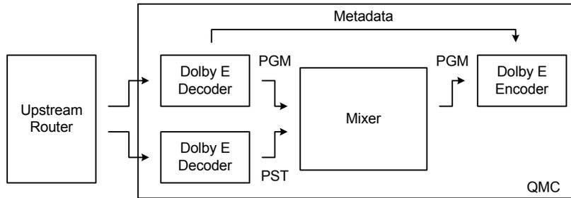
All 8 channels are then processed internally and output as two groups of four audio signals. In this configuration input AES and Dolby E audio can be mixed, and voiceovers inputs used as normal.
