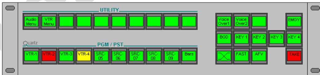
The buttons on this style of panel are LCD types that display text provided by the control system. This allows buttons to be re-configured for different applications to suit customer preferences. Typical operation involves selecting a preset source, and then selecting the transition type, speed of transition, and then pressing the TAKE button. The button colour changes to show status.
