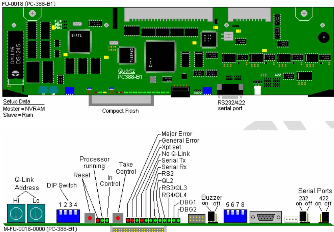
The FU-0018 processor has four RS232/422 serial ports and two Q-Link ports.
