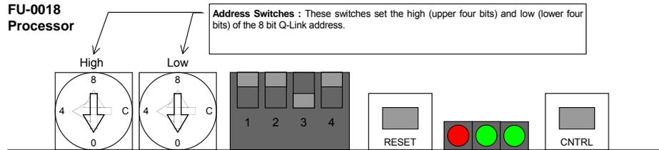
The reset switch must be pressed after changing the address switch.
