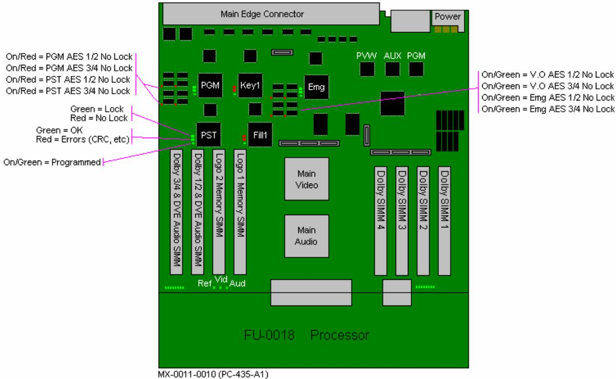
The QMC-2 main module has 5 HD/SD inputs for PGM, PST, KEY/FILL 1 and Emergency, outputs for PGM, PVW and AUX, and all the AES inputs and outputs. A daughter module can be added to give five additional inputs of KEY/FILL2, KEY/FILL 3, and DVE background.
