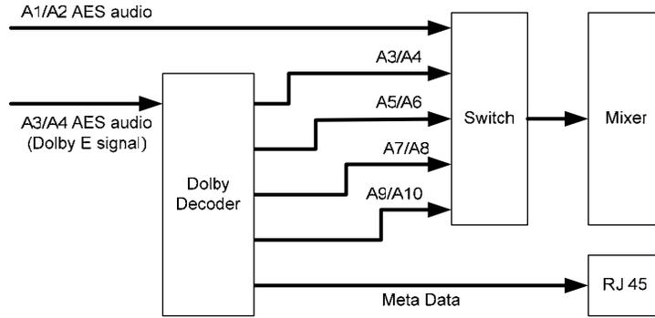
The Dolby E decoder in the QMC will maintain the order of the audio tracks as they had been set prior to the encoder. However, the track numbering can be changed if required as shown in the diagram below.
