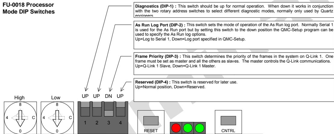
The reset switch must be pressed after changing the DIP switch.
