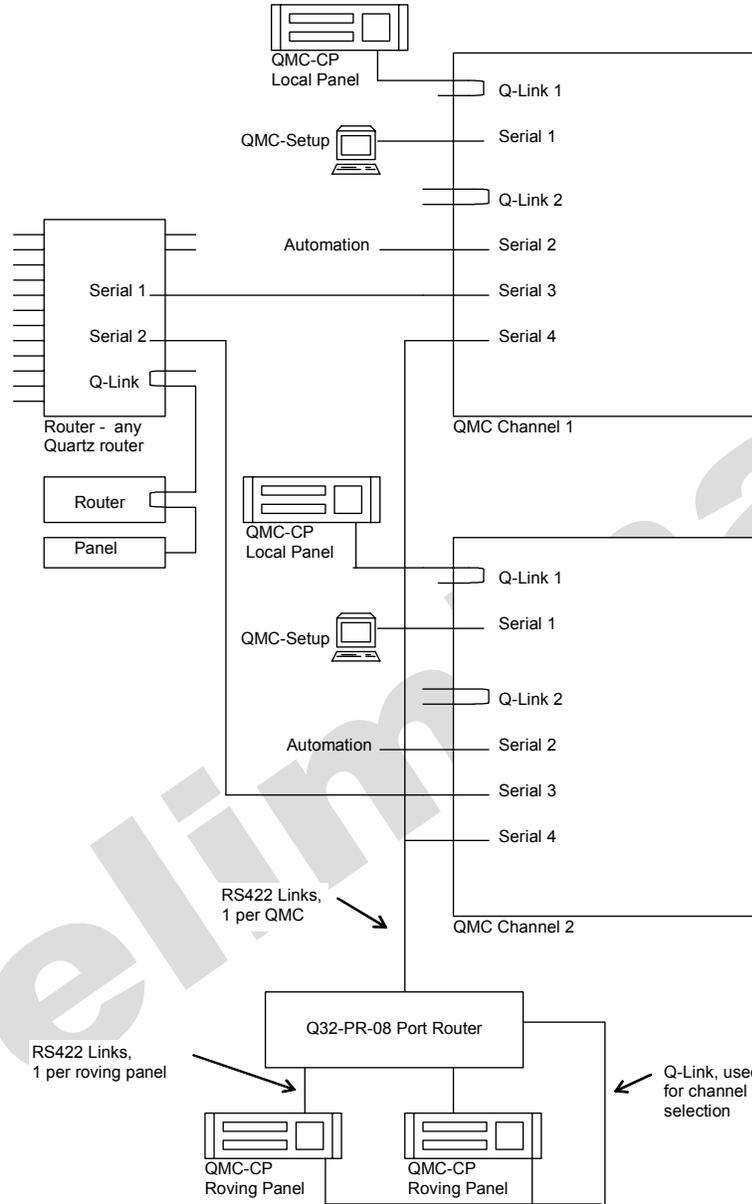
**2.3.4. Configuration D: 3-62 Channels, Small Up-stream Routers, 0 or 1 Roving panel**
