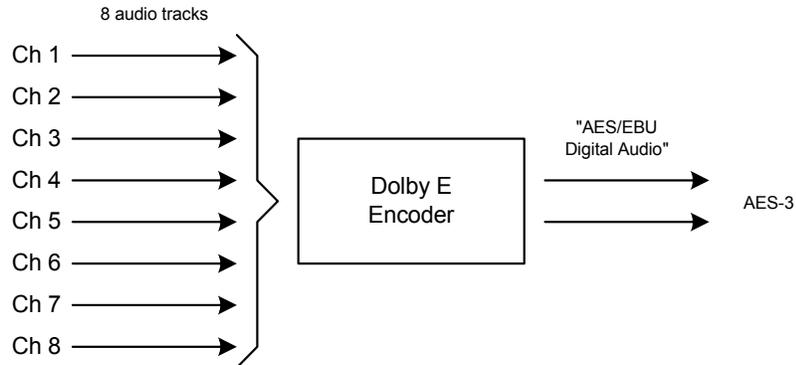
This enables distribution via a single AES-3 pair or recording on two audio tracks of a digital video tape, to create a standard exchange format for sound with picture. Dolby E encoded audio is designed to withstand ten or more of the encode/decode cycles typically required during the distribution phase of DTV programs.
