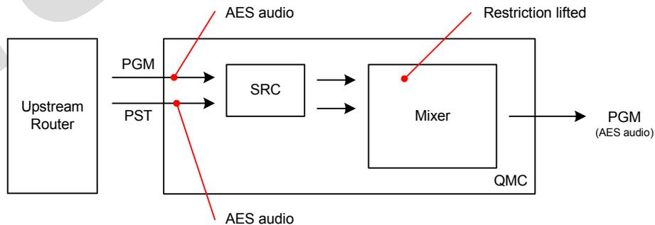
In the Bypass mode transitions between stereo AES audio and Dolby E are possible, but only as cuts. Since there is no Dolby E decoding metadata preserved on all Dolby E streams.
