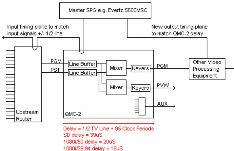
If input timing is out by more than +/-1/2 line then video artefacts will be present. As an example Closed Captioning can be moved down one line if the input video is delayed by more than 1/2 line (assuming ITW register is set to zero, see below).
