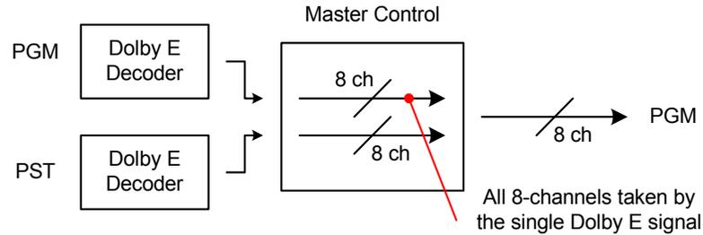
However, within a 16 channel system, such as the QMC-2, 8 of the 16 channels are still available. These channels can be used to carry a second Dolby E signal or 8 additional and independent AES/EBU audio signals, such as a separate language track, natural sound etc.
