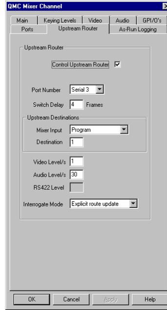
If Q-Link is being used, select the Ports tab and configure Q-Link-2. Remember to add the Q-Link address of the QMC-HD/SD as specified in the router setup. This address is entered into the first Protocol Data Byte **but must be entered as a decimal number** (18 hex = 24 decimal).
