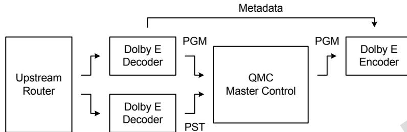
If the signal is being fed to through a link directly to a transmitter then the final encoder may be a Dolby Digital (AC-3) encoder rather than a Dolby E encoder.
