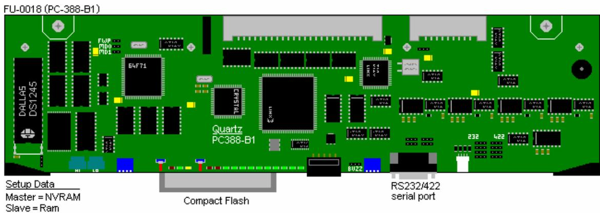
The System Software flash memory device contains all the operation firmware defining how the QMC will operate. The NVRAM stores current settings, setup data, etc.
