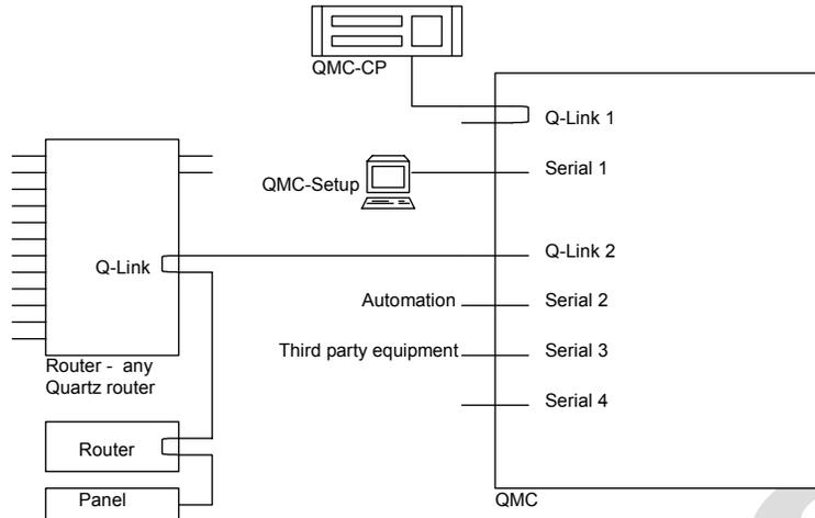
In the example above Q-Link 1 is used for the QMC-Link to QMC control panels. Serial 1 would normally be used for downloading from a PC running the QMC Setup program. Q-Link 2 is being used to control an upstream Quartz routing system. Only two routers and one control panel are shown because the upstream router Q-Link must not have more than four devices connected.
