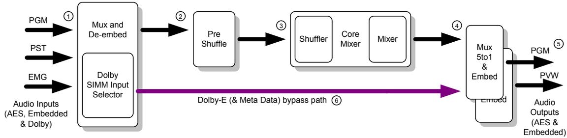
The diagram above shows the audio path taken through the QMC-2 of an AES and embedded audio feed with the Dolby E bypass selected.
