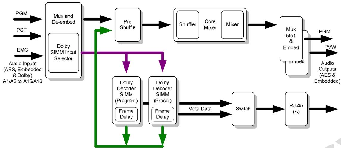
The audio path is identical to the previous example shown but with the addition of two Dolby E decoders<sup>7</sup>. These decoders are optional and are fitted to the main QMC-2 module.
