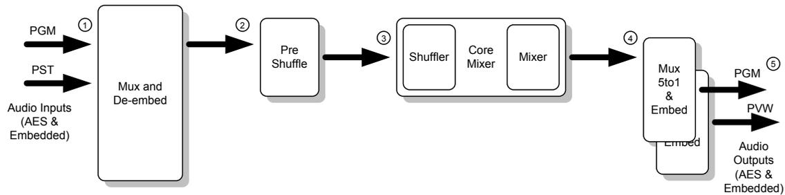
The above diagram shows the audio path taken through the QMC-2 of a non Dolby E AES and embedded audio feed.
