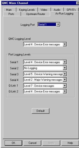
The As-Run log would normally be configured to log to port Serial-1 as this usually has the QMC-Setup PC connected. As-Run logging should normally be turned off. Do not set an unnecessarily high level of logging, as this will eventually slow down the QMC operation.
