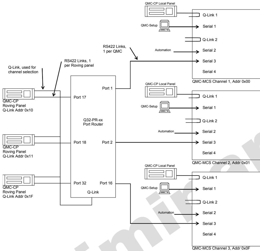
Roving panels and QMC Channels must be connected to specific ports on the port router, defined by their Q-Link address.
