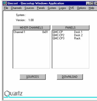
The Switcher Channels section lists all the QMC Switchers being used in a multi-channel system. A single channel system will only show one QMC channel. Any manual QMC-CP control panels are shown under the panels section.
