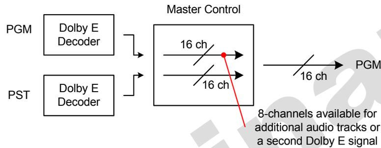
For example, within an embedded SDI feed additional audio tracks can be added upstream of the QMC-2, as well as added into the Program path via the Voiceover facility. These additional audio tracks are then processed through the QMC and carried out to its Program output.
