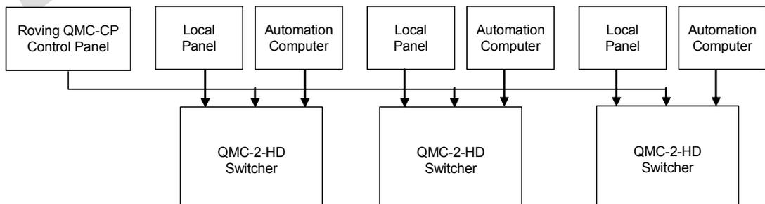
In a multi-channel system each QMC channel is independent of other channels. Each Automation computer has its own link to the QMC channel that it is controlling. In this way no single point of failure can stop transmission control of the majority of Switcher channels.
