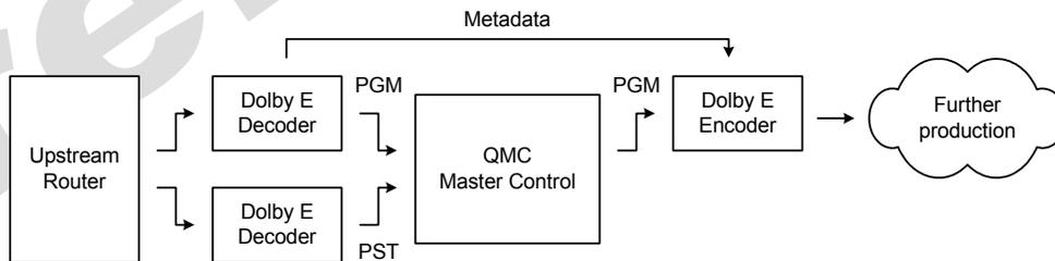
With this arrangement all transitions are possible in the QMC-2, including voiceovers. During a dissolve the meta data will continue to come from the outgoing source until the end of the transition, at which point it will cut to the meta data from the incoming source.
