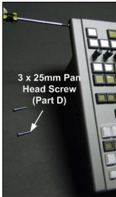
Figure 3-4: Securing the Top Guide Rotation Lock – Right Side
