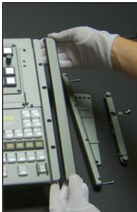
Figure 2-2: Remove the Protective Covering from the Right Side
