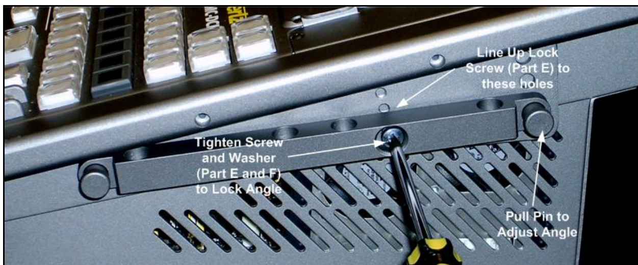
Figure 3-8: Adjusting and securing the angle
