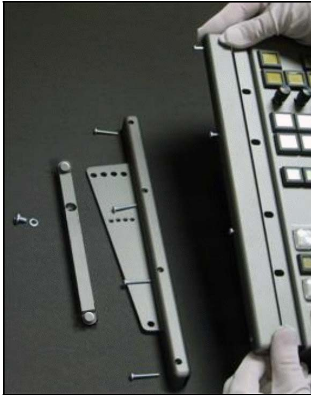
Figure 2-3: Remove the Protective Covering from the Left Side
