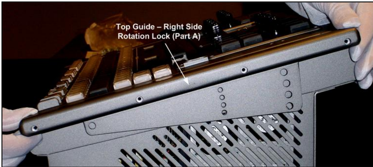
Figure 3-1: Attaching the Top Guide Rotation Lock – Right Side
