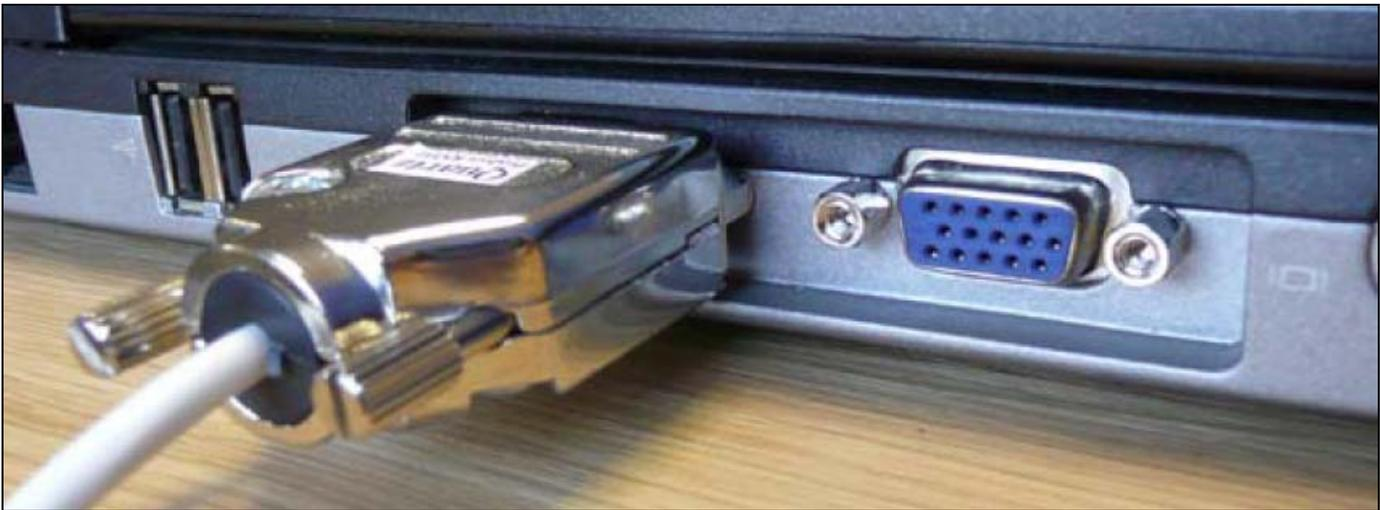
**Figure 1-5: Quartz Serial Cable Connected to the Serial Port Mounted on the PC Rear**
