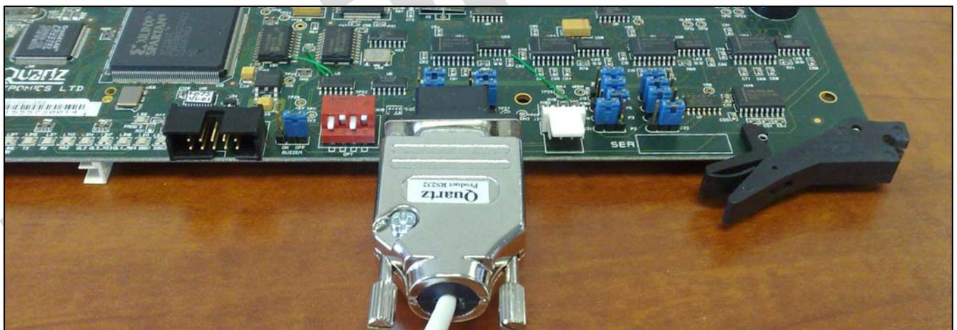
Figure 1-4: Quartz Serial Cable Connected to the Front Serial 1 Port of the QMC-2
