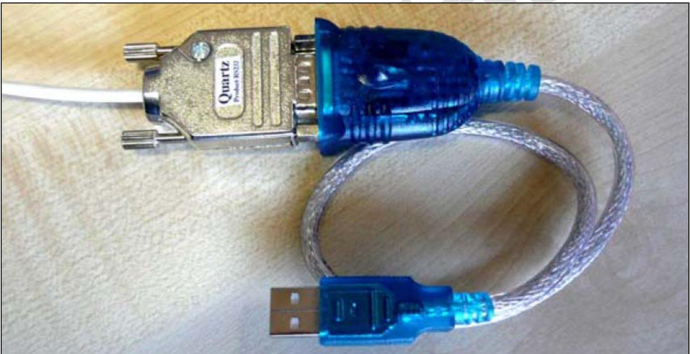
**Figure 1-6: Serial to USB Converter**
