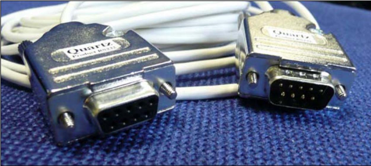
**Figure 1-2: Quartz Serial Cable Ends**
