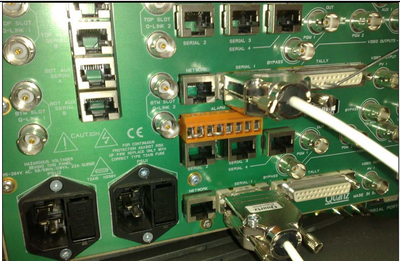
Figure 1-3: Quartz Serial Cable Connected to the Serial Port 1 of the QMC-2
