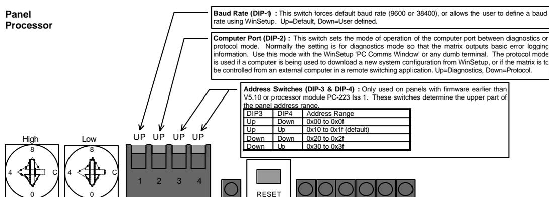
The reset switch must be pressed after changing the DIP switch.
