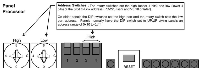
The reset switch must be pressed after changing the address switch.
