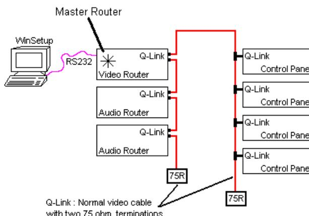
In medium sized systems it may be more suitable to have several Q-Links on the master frame and to wire off in different directions. This requires a CI-0004 module in the master router. Only Q32 routers and above have the extra BNC connectors to support a CI-0004.
