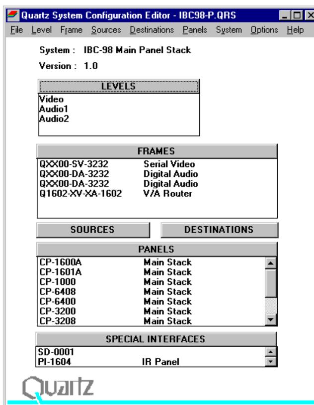
If you are generating a system configuration from new then some of the menu's and functions are greyed out (not available). This is deliberate to 'lead you through' the functions that need to be set up. Carry out the following functions to configure your system.
