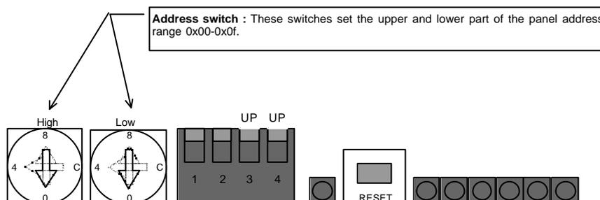
Panels with identical hardware can be exchanged in a system by transposing the Panel Addresses. Note that these instructions only apply to current control panels fitted with PU-0006 (PC-223 Issue 2).
