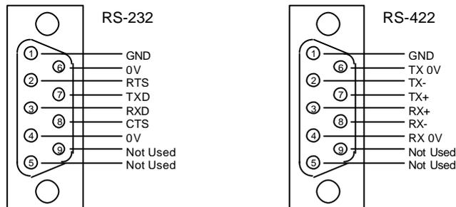
The cable between the PC and the router (RS232) only needs to use TX, RX, and GND as shown below.
