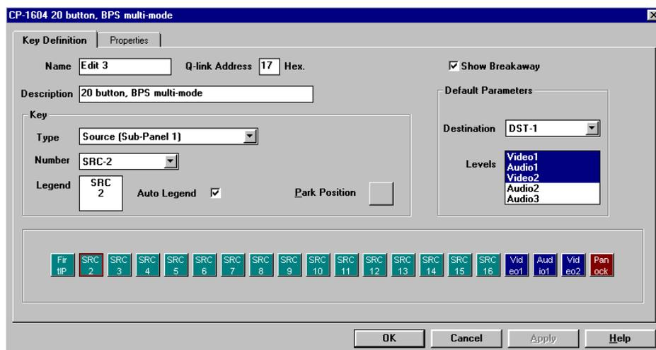
Each button can be programmed by selecting the button and then editing the functions in the key section. Each panel should also be given a name for later identification, EDIT 3 in this example. The Q-Link address will be allocated automatically by the program but can be edited if required. The default parameters control how the panel will function at power up, in this example the panel will always control DST-1 to start with. Now add any further panels that the system will need.
