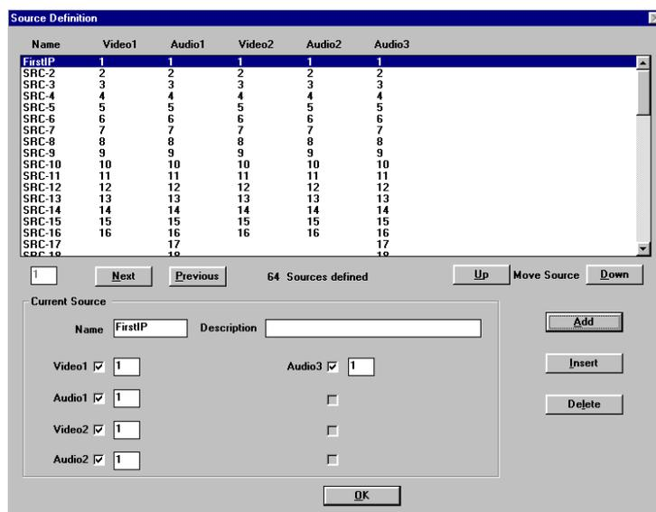
If you want to edit a name now then select one row from the list of names in the upper part of the screen, the details appear in the lower part of the screen. From here you can edit the name and decide which signal levels that name will control when selected on a control panel.
