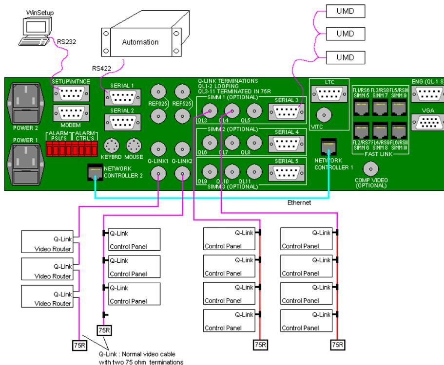
As a system design guide the SC-1000 should be considered when the router grows above 128x128 single level or has more than 10-15 total Q-Link devices. See section 6.10 for further information on the SC-1000.
