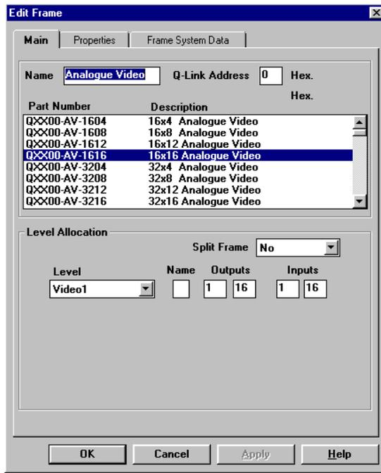
Router frames have to be 'attached' to the router level that they are to follow, and this is set in the level allocation section in the lower half of the screen.
