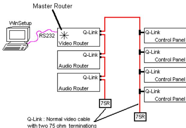
This daisy chain method ensures the best transmission quality of the control signals down the cable. Short cuts that might save cable, such as running stubs to some panels, are not recommended as this may cause data errors under certain circumstances. The maximum cable length is shown in the Technical Specification in Section 2 of this manual.
