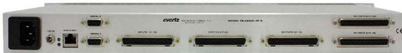
Figure 1-4: Rear Panel View of the TR-4800E with the +BP16 option
