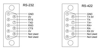
Figure 2-10: RS232/422 Connecting to the Router
