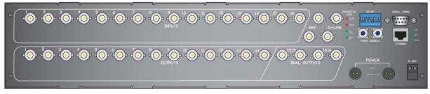
Figure 2-4: Rear View of Topaz QT-1616H Router
