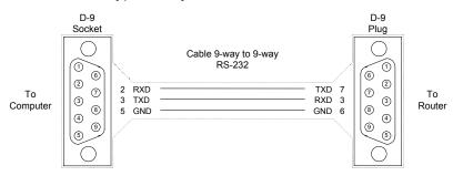
Figure 2-11: RS232/422 Connecting to the Computer
