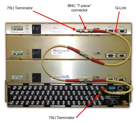
Figure 3-1: Q-LINK to Three Remote Control Panels (shown on Topaz Router)
