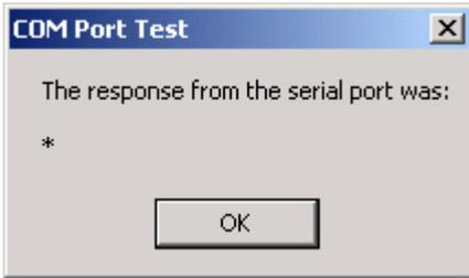
If the encoder is not properly connected, the dialog box will state that the serial port has timed out. This error can also display if the proper bit setting and parity is not set correctly.
