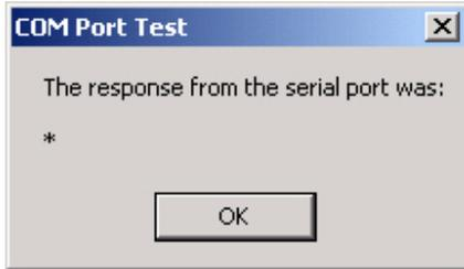
If the encoder is not properly connected, the dialog box will state that the serial port has timed out. This error can also display if the proper bit setting and parity is not set correctly.
