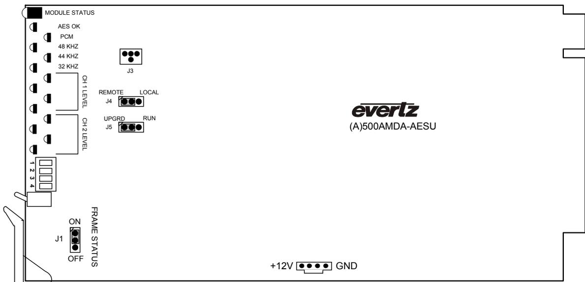
**Figure 2: Location of UPGRADE Jumper on 500AMDA-AESU Boards**
