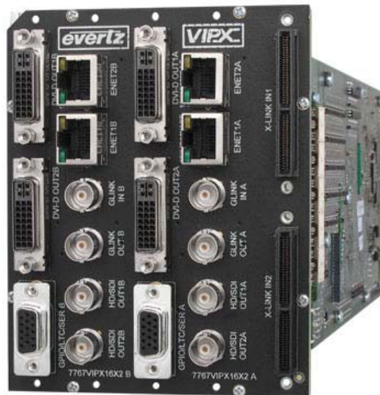
Figure 2-14: VIPX-RP2 Rear Plate
