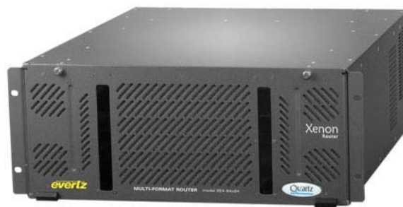
Figure 2-1: Xenon 4RU – 64x64 Router
