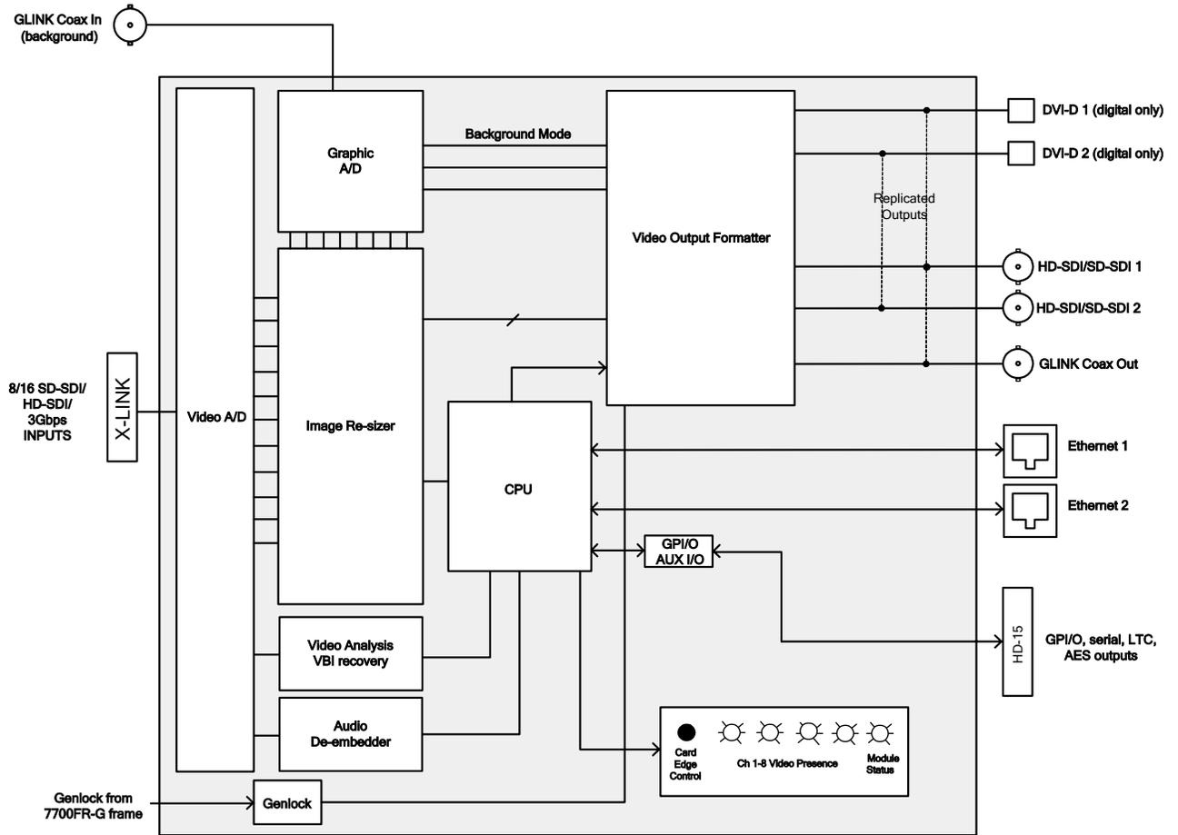
Figure 5-8: 7867VIPX8x2/16x2/32x2 Block Diagram
