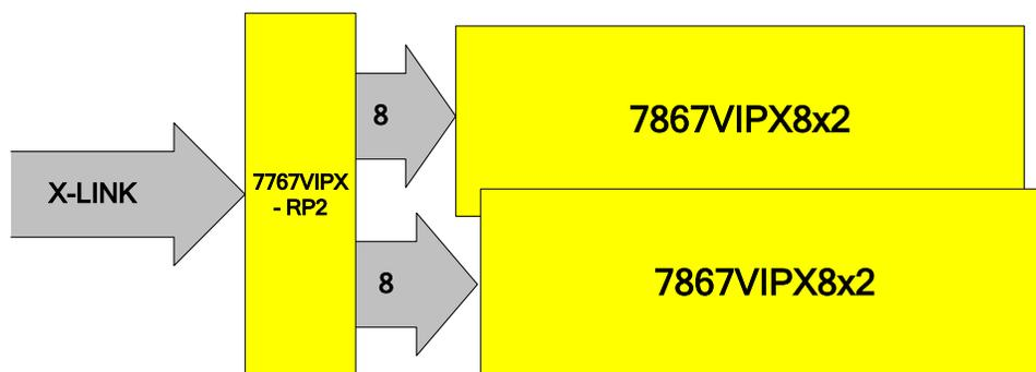
**Figure 2-17: Distribution of X-LINK connections to the 7867VIPX8x2**
