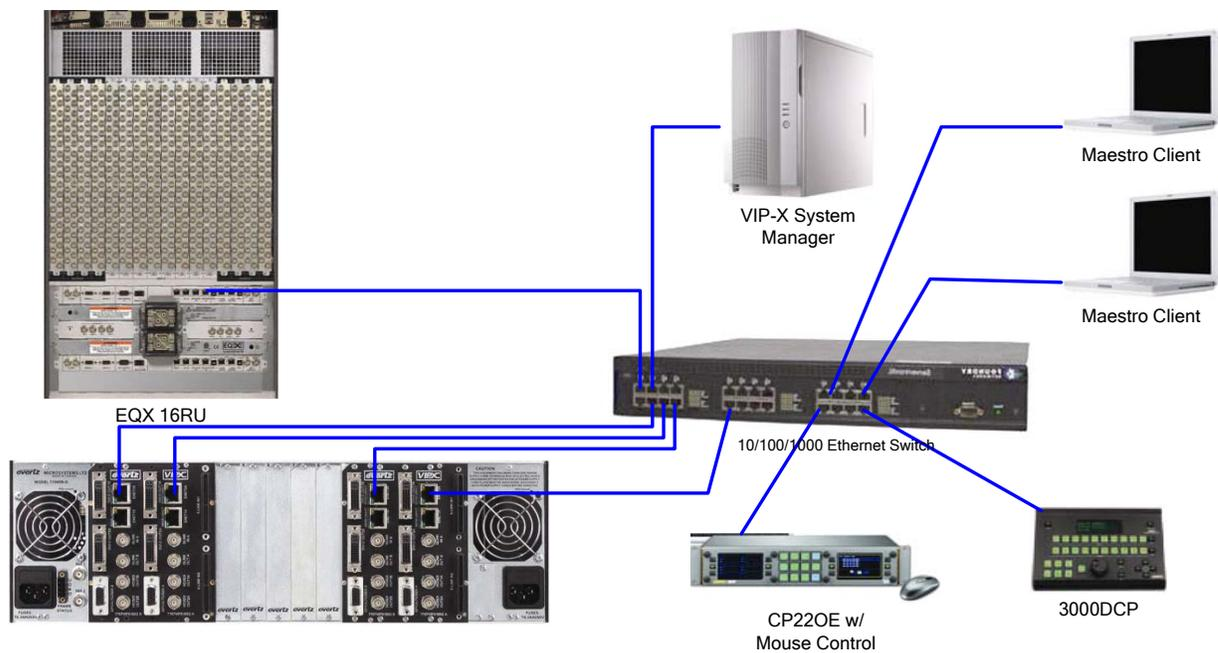
**Figure 4-2: Network Connectivity Diagram – EQX 16RU Router**
