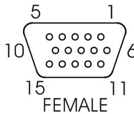
**Figure 5-6: 7867VIPX16x2/8x2 HD-15 General Purpose Pin-Out**
