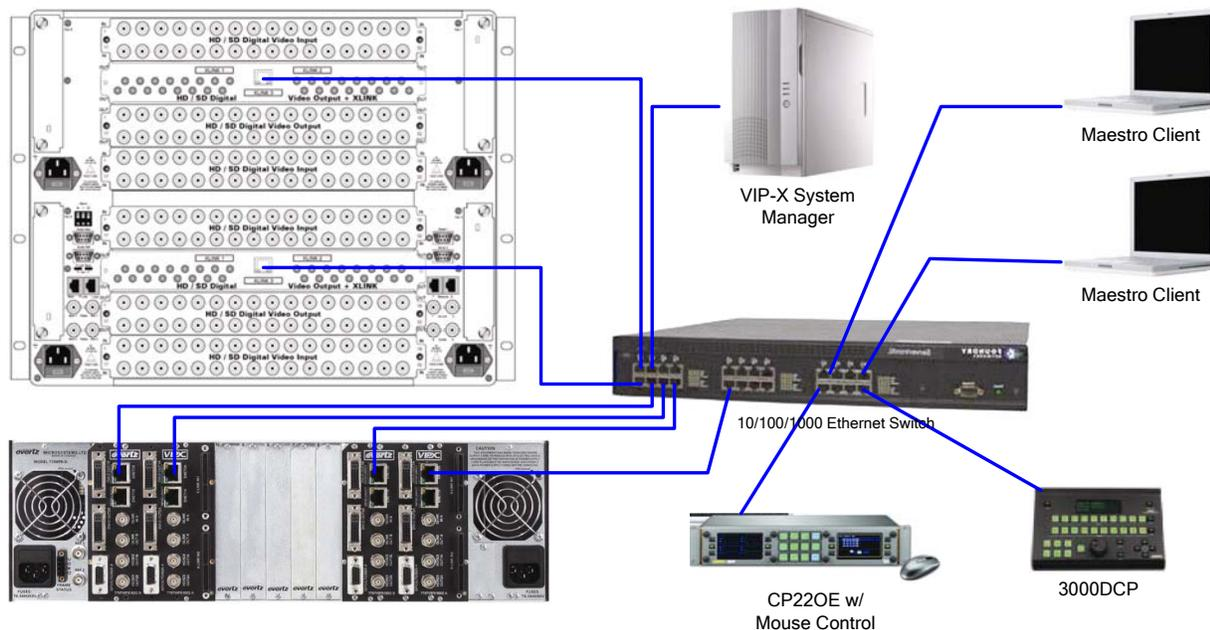
Figure 4-1: Network Connectivity Diagram – Xenon Router
