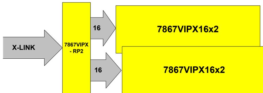
**Figure 2-16: Distribution of X-LINK connections to the 7867VIPX16x2**
