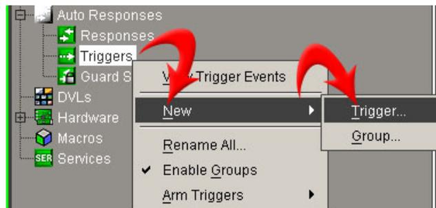
**Figure 3-1: Using the Navigation Tree to Create a Trigger**
