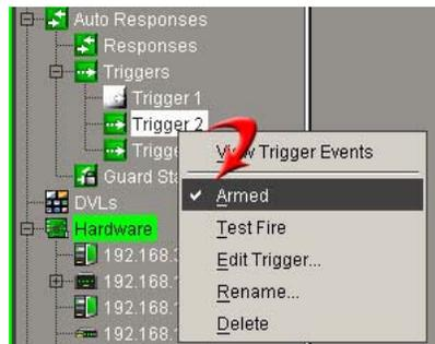
Figure 3-15: Controlling the Armed State for a Trigger
