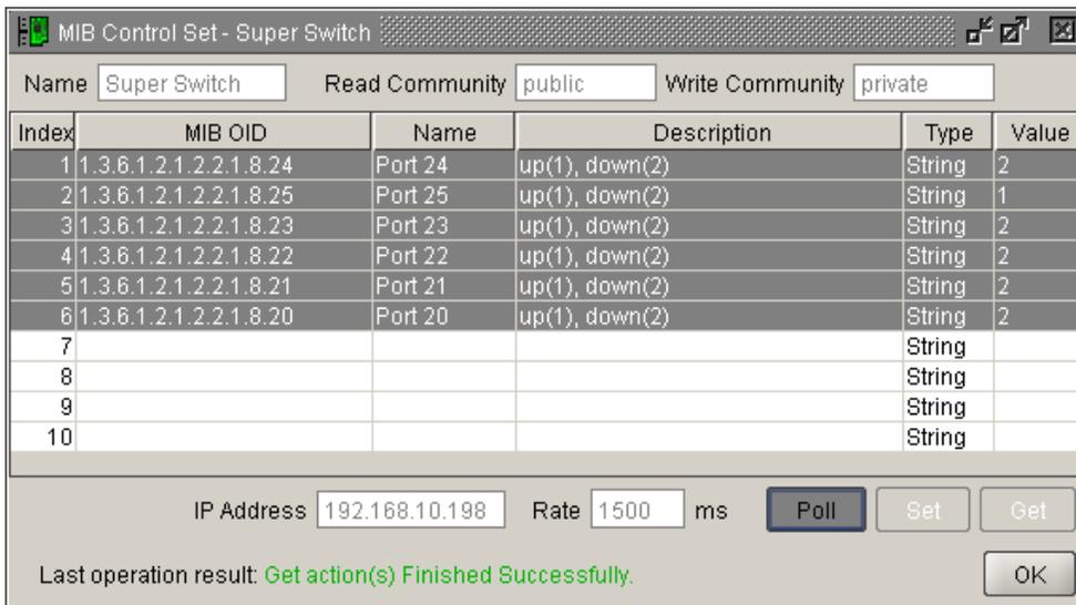
Figure 6-23: Super Switch MIB Control Set in Action
