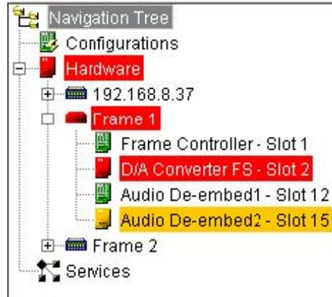
Figure 5-2: Example of an Alarm Condition
