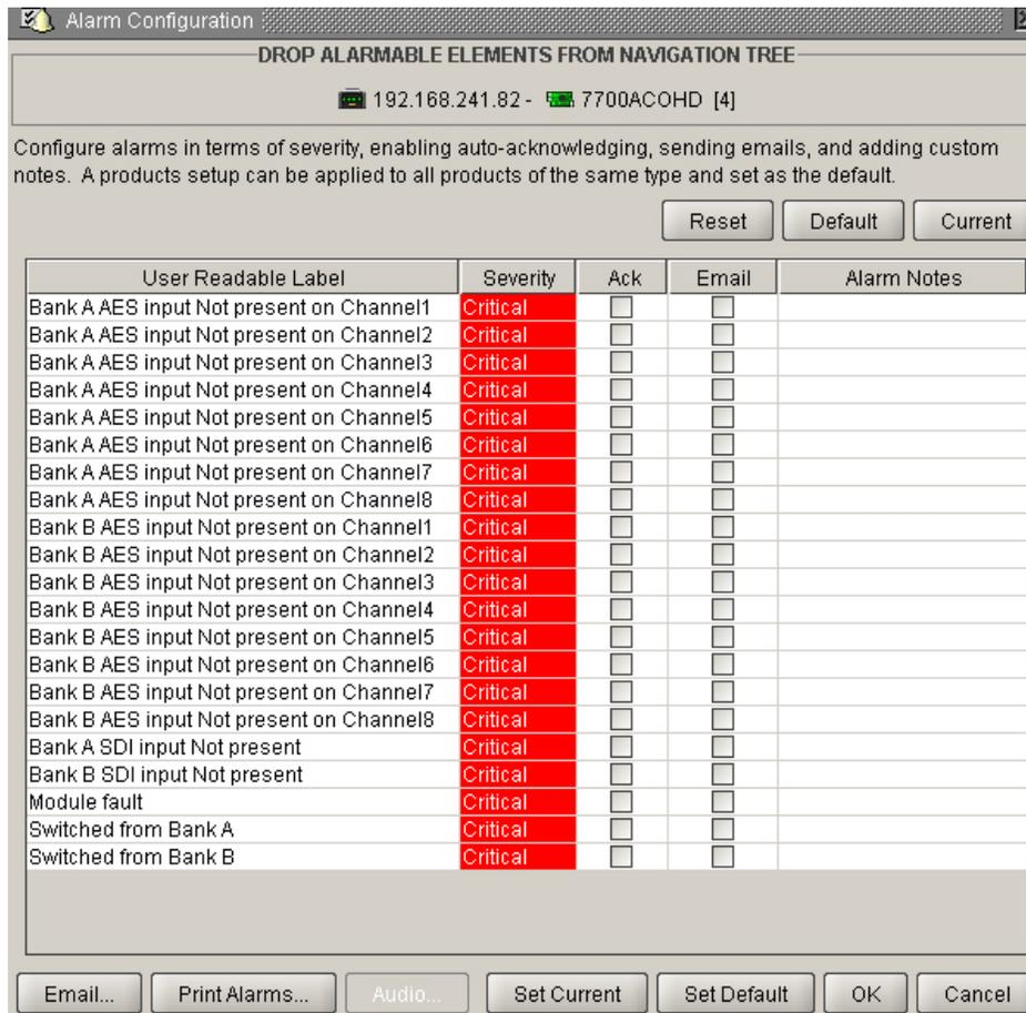
Figure 5-6: Alarm Configuration Window
