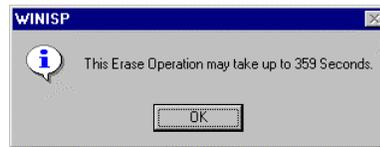
This is a worst case timing and you should not be alarmed if the erase function is much quicker than indicated. After erasing you should verify the erase with a BLANK CHECK.
