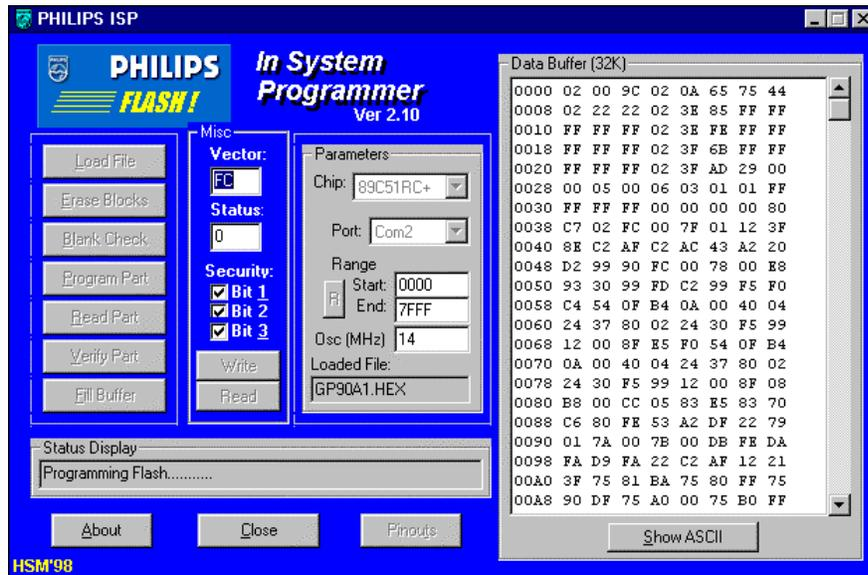
Power down and then re power the unit and you will have successfully upgraded the software. If you used the DIP switch method to initiate programming, remember to restore DIP switch 7 to its original position.
