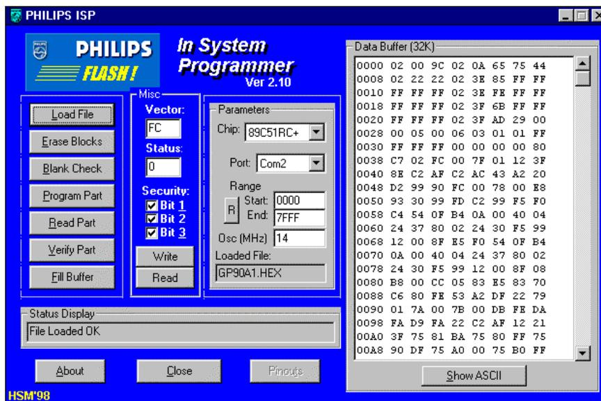
Then press the PROGRAM PART button and the new software will be downloaded into the unit. When finished verify the programming using the VERIFY PART button. If the part verifies then you are done.
