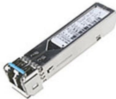
Figure 5-26: SFP Transmitter Module
