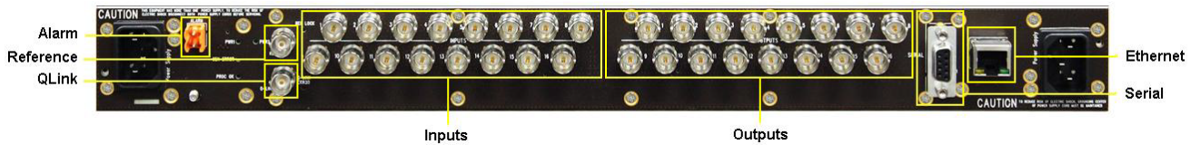
Figure 4-10: Rear Communication Connections on the EQT-1616 and EQT-1604
