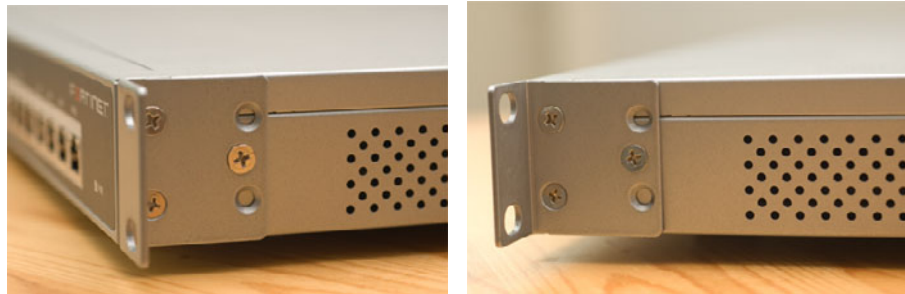
Figure 351: Installed 2U mounting brackets
