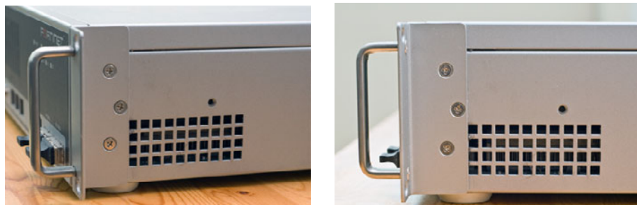
Figure 351: Installed 2U mounting brackets
