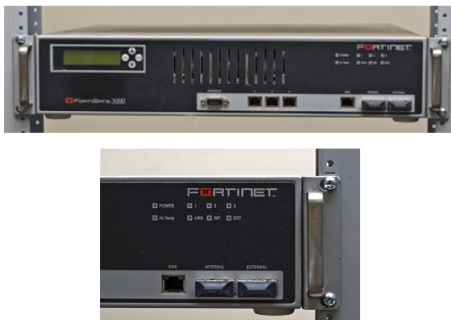
Figure 353: Mounting a 2U FortiGate unit in a rack
