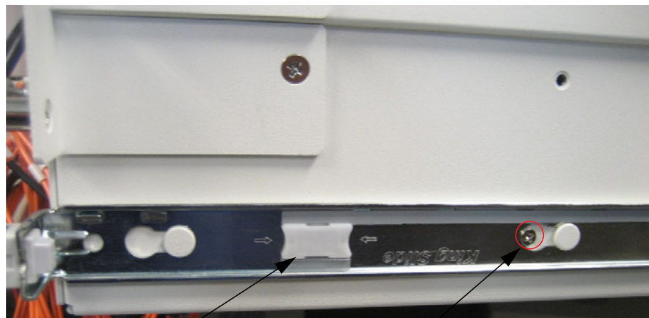
Figure 356: Optional screw hole for additional support.
