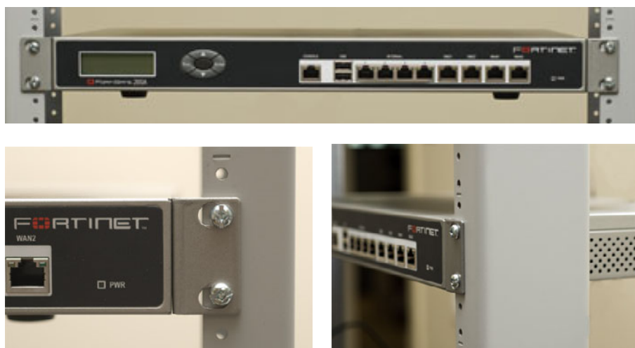
Figure 353: Mounting a 2U FortiGate unit in a rack
