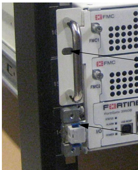
Figure 362: Location of locking mechanism on rail and screw hole in front handle.
