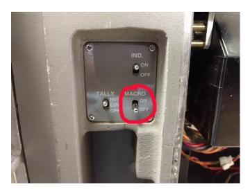
2- F.f switch on the left side behind the shroud need to be in remote
