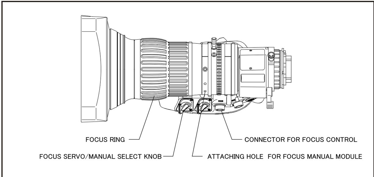
Focusing can be done by directly rotating the focus ring by hand. Rotate the focus ring clockwise from the camera side to focus on an object on the near side.
