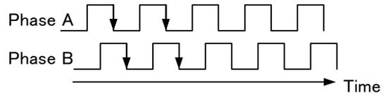
(2) Waveforms of Zoom Encoder Output Signals
