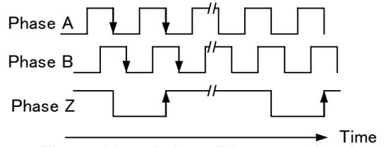
\* The position of phase Z is not regulated to that of phase A or B.
