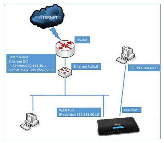
Figure 13: UCM6102 Network Interface Method: Switch
