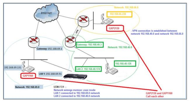
The following diagram shows a sample application of static route usage on UCM6104.
