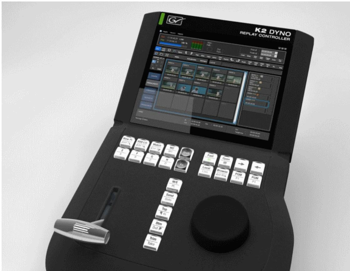
Many of the functions of the K2 Dyno S Replay Controller are operated from the large touch screen. Three key elements of the touch screen are Tabs, Slots, and Bins.
