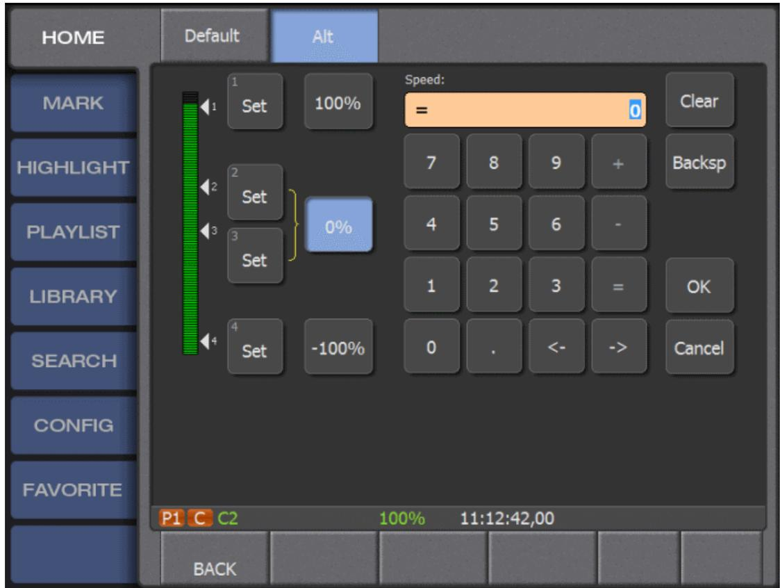
The four **Set** boxes set the custom speeds on the path of the T-bar, as indicated by their position on the graphic range bar.
