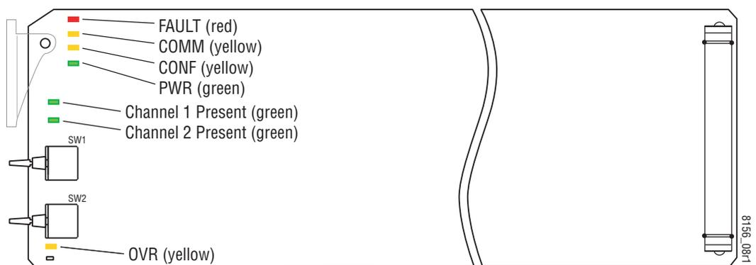
**Note** The yellow **COMM** and **CONF** LEDs are used for the module location function that is enabled using the GUI. The module location function causes these LEDs to flash concurrently three times followed by an off state of 900 ms duration. The locate mode can be turned off by toggling the paddle switch on the module.
