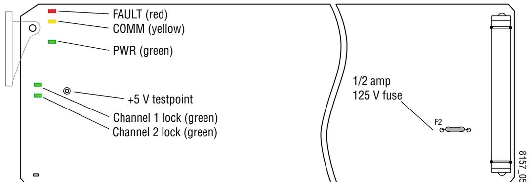
A red FAULT LED indicates an error situation and, with the previously described LEDs, can indicate the operational conditions presented in [Table 1 on page 12](#). The table describes LED indications and the signal input/output conditions that are indicated.
