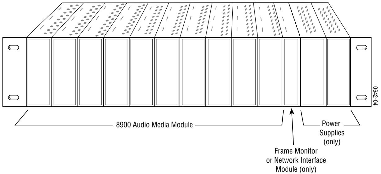
8900 module slots are interchangeable within the frame. There are 10 three-terminal connectors and 4 BNC connectors in each slot's I/O group. The functional assignment of each connector in a group is determined by the module that is placed in that slot. The maximum number of media modules an 8900 frame can accept is ten. Figure 2 illustrates the rear connector plate for an 8900 Series frame.
