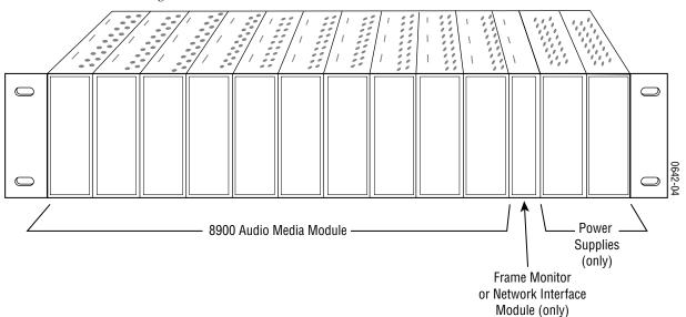
8900 module slots are interchangeable within the frame. There are 10 three-terminal connectors and 4 BNC connectors in each slot's I/O group. The functional assignment of each connector in a group is determined by the module that is placed in that slot. The maximum number of media modules an 8900 frame can accept is ten. Figure 2 illustrates the rear connector plate for an 8900 Series frame.
