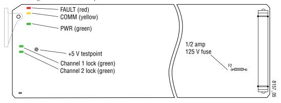
A red FAULT LED indicates an error situation and, with the previously described LEDs, can indicate the operational conditions presented in Table 1 on page 12. The table describes LED indications and the signal input/output conditions that are indicated.
