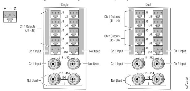
Figure 3. 8912RDA Single and Dual Channel Input/Output Connectors
