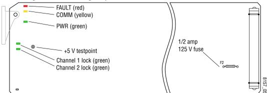
Figure 6. Fuse and Voltage Testpoint Locations
