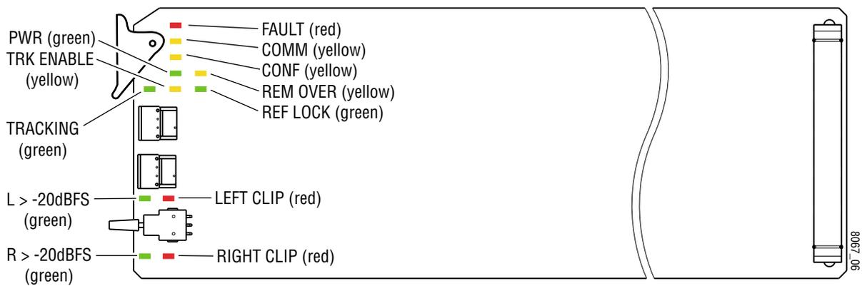
A red FAULT LED indicates an error situation and, with the other LEDs, can indicate the operational conditions presented in [Table 4](#). The table describes signal output and LED indications for various input/reference combinations and user settings.
