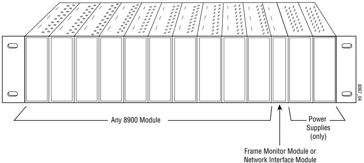
8900 modules are interchangeable within the module cells. There are 10 BNC connectors in each cell's I/O group. The functional assignment of each connector in a group is determined by the module that is placed in that cell. The maximum number of modules an 8900 frame can accept is ten. Figure 2 illustrates the rear connector plate for an 8900 Series frame.
