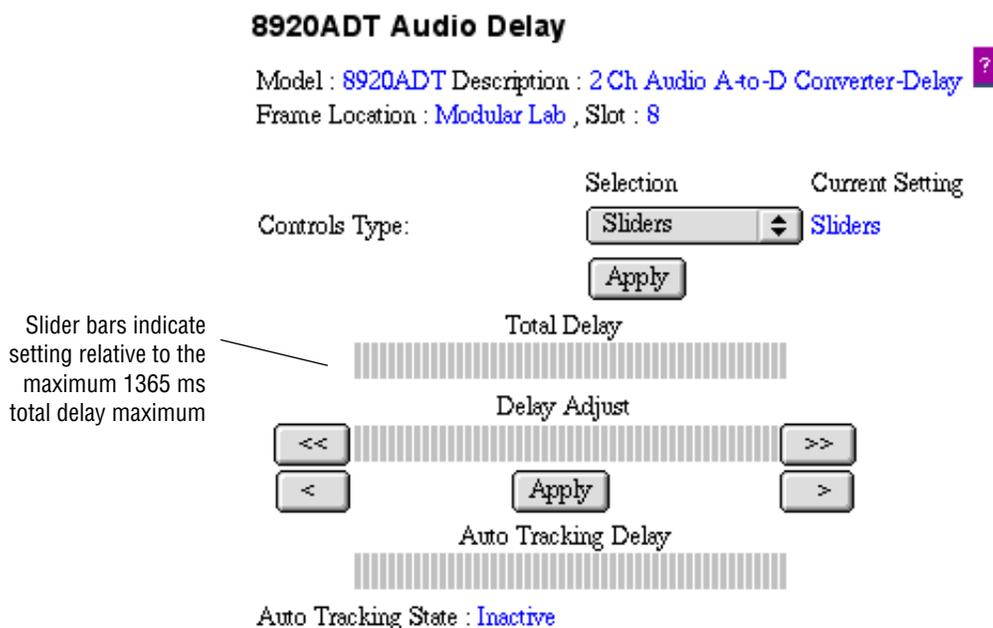
The slider mode provides a view of the delay setting relative to the module's maximum 1365 ms.
