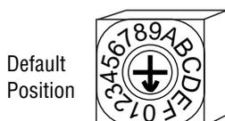
Set the Mode Rotary Switch at the front of the module to the Default position marked 0 as shown at left. The Default position will put each channel output into a normal mode with no phase inversion, channel swapping or summing.
