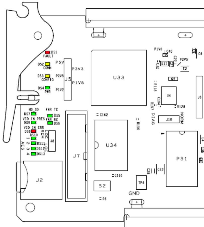
A continuous FAULT LED on (red) indicates an error situation and, when noted with the other indicator LEDs, can indicate a specific problem area. [Table 3](#) describes signal output and LED indications for the various input/reference combinations.
