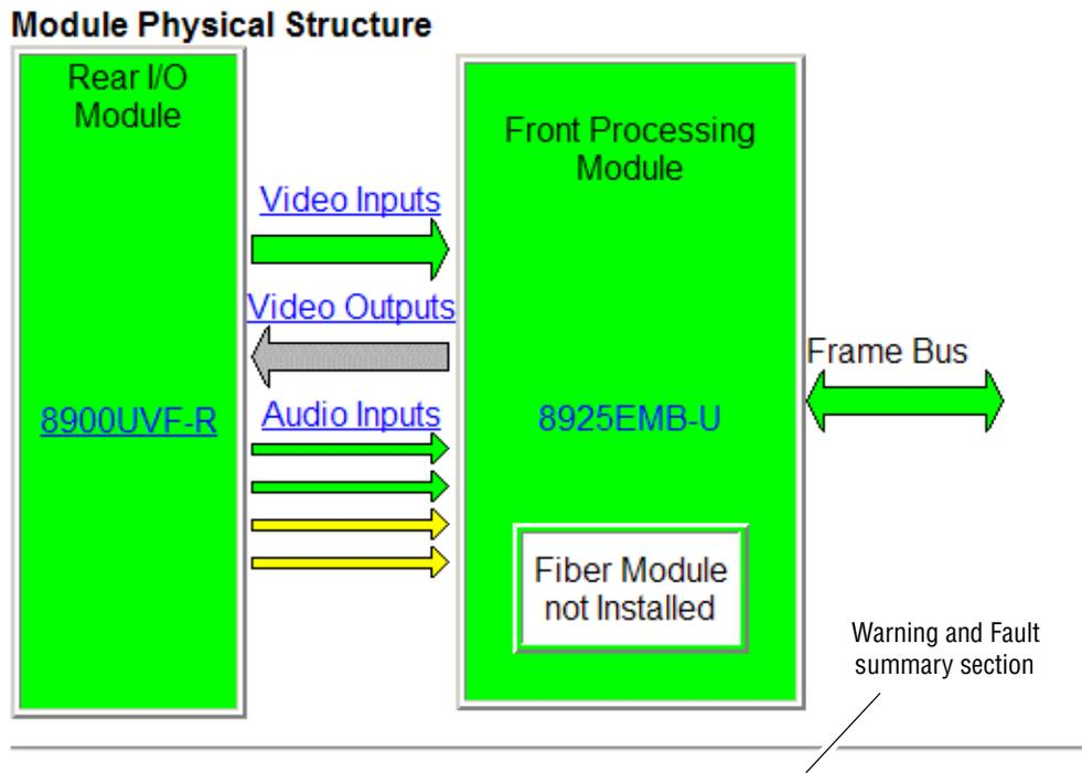
Fiber Module is not installed
