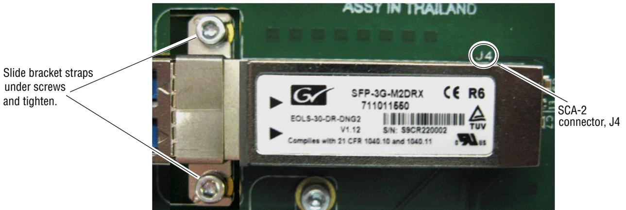
Now install the Fiber Channel 3 and 4 fiber cable assembly from the SFP device to the rear connector as described below.
