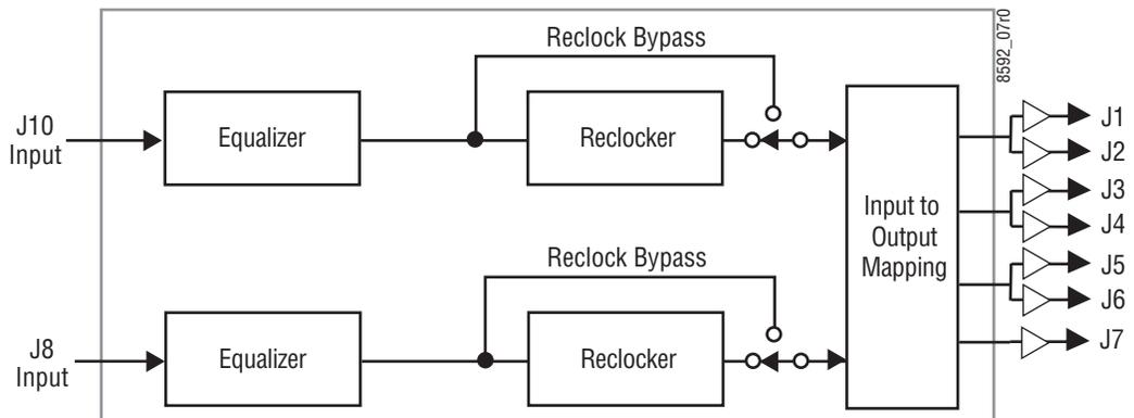
A block diagram of the 8943RDA-DFR with a dual receiver fiber optic submodule installed is shown in [Figure 44](#).
