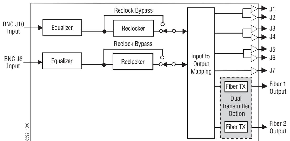
A block diagram of the 8943RDA-DFR with a transceiver fiber optic submodule installed is shown in [Figure 46](#).
