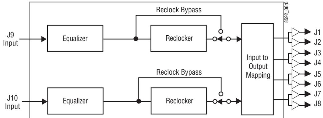
A block diagram of the 8943RDA-DFR without fiber optic submodule installed is shown in [Figure 43](#).
