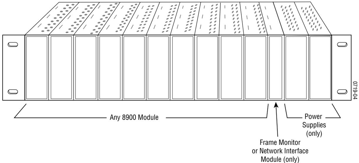
8900 modules are interchangeable within the module slots. There are 10 BNC connectors in each slot's I/O group. The functional assignment of each connector in a group is determined by the module that is placed in that slot. The maximum number of modules an 8900 frame can accept is ten. [Figure 2](#) illustrates the rear connector plate for an 8900 Series frame.
