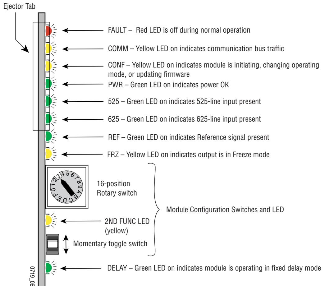
A red FAULT LED indicates an error situation. When in Frame Sync mode, the 525 or 625 LEDs will blink if the reference signal input line standard does not match the video input standard.
