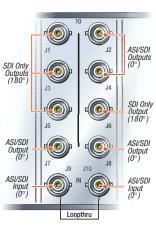
The 8931 digital video fanout distributor amplifier is designed for distributing all major serial digital video formats. It is especially suited for short runs of recently reclocked signals where jitter is not a problem.
