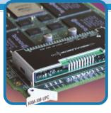
Designed for HD upconversion of SDI video with or without embedded audio, our KAM-XM-UPC module provides uncompromised, high-guality performance in a cost-effective platform. It features Teranex de-interlacing, 3:2 detection, and detail-enhancement technologies combined with powerful array processing provide the best imaging solution. It also supports our Newton Ethernet-based modular control system. NetConfig configuration tools, and NetCentral SNMP-based monitoring software.
