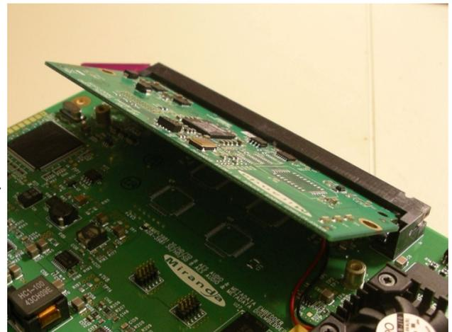
4. Pull the module out of the socket
