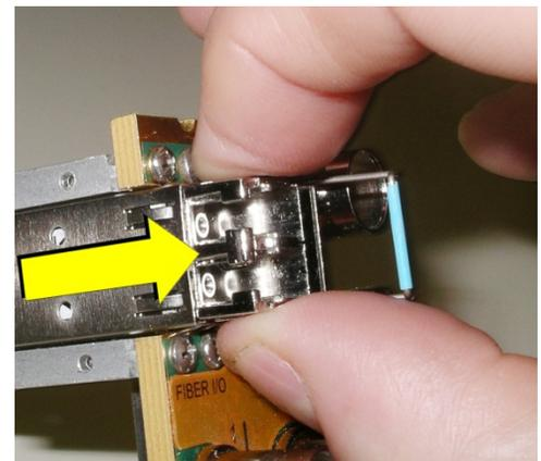
3. Insert a dust plug into the SFP module.
