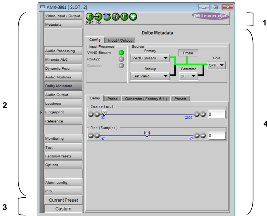
Figure 5.1 AMX-3981 iControl graphic interface window
