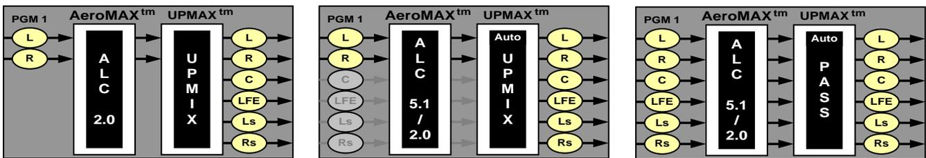
Note: The MOD-LA-ALC-X-YYY works with PCM audio. If non-PCM audio like Dolby E or Dolby Digital is fed to the module, it will be ignored and silenced to prevent interference with the other PCM audio channels.
