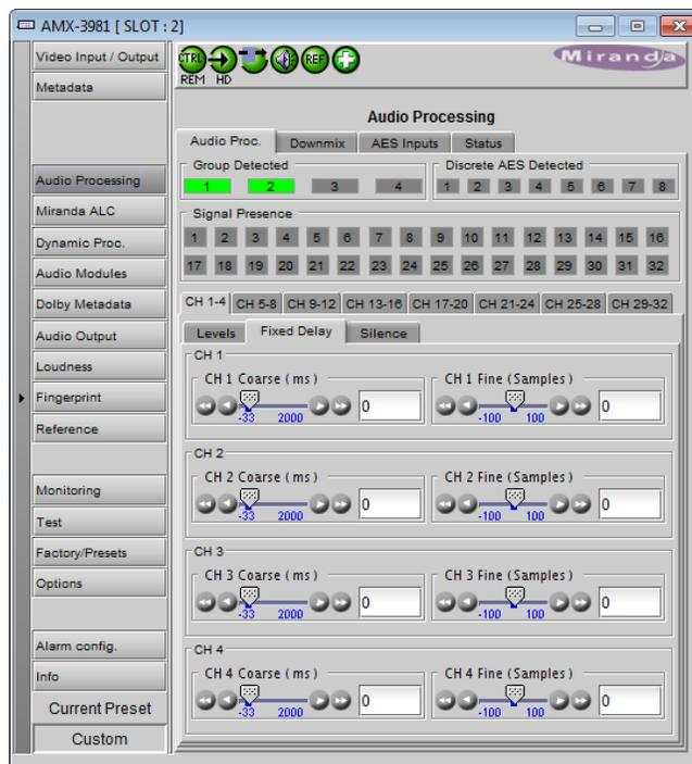
Figure 5.14 Audio Processing – Channels - Fixed delay
