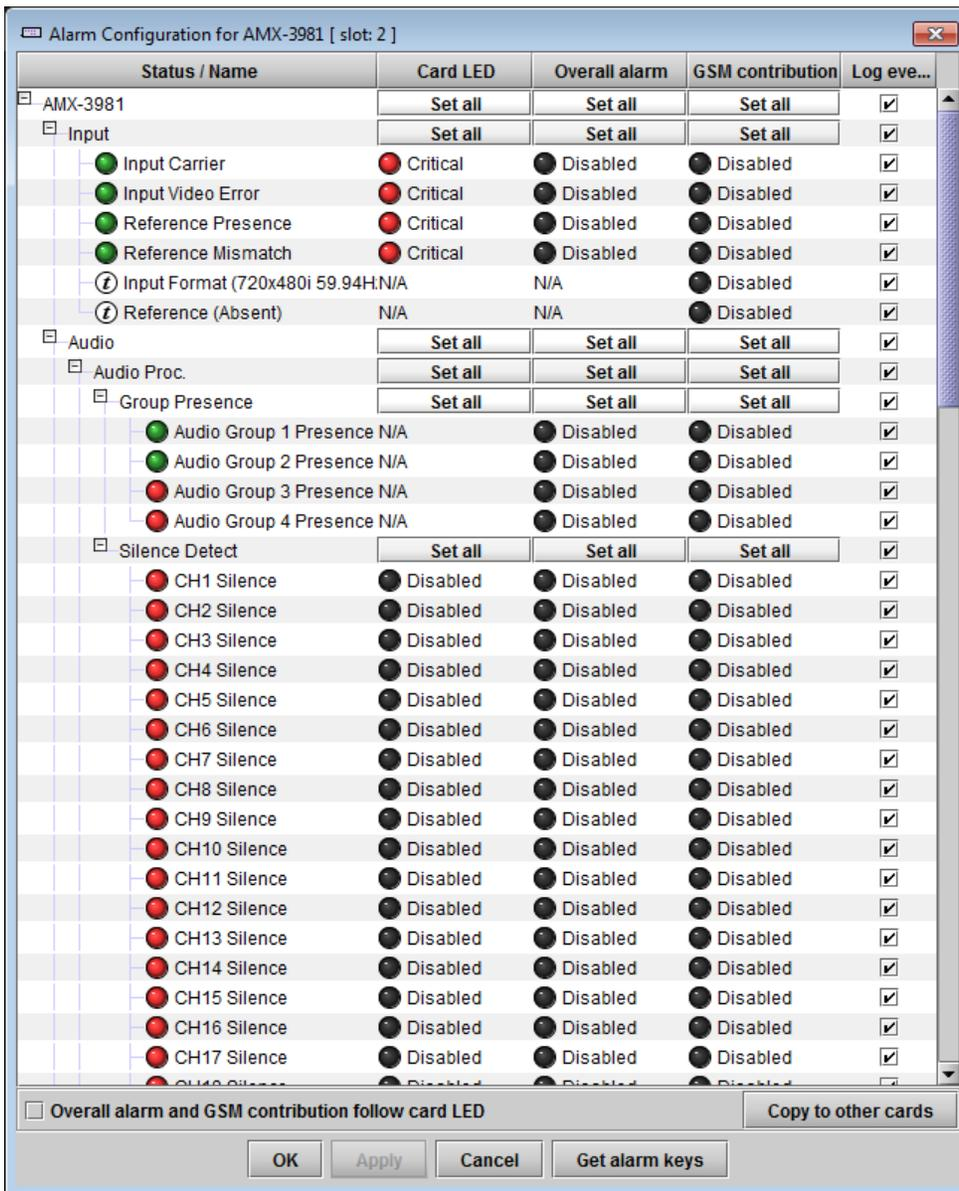
Figure 5.64 Alarm Configuration panel
