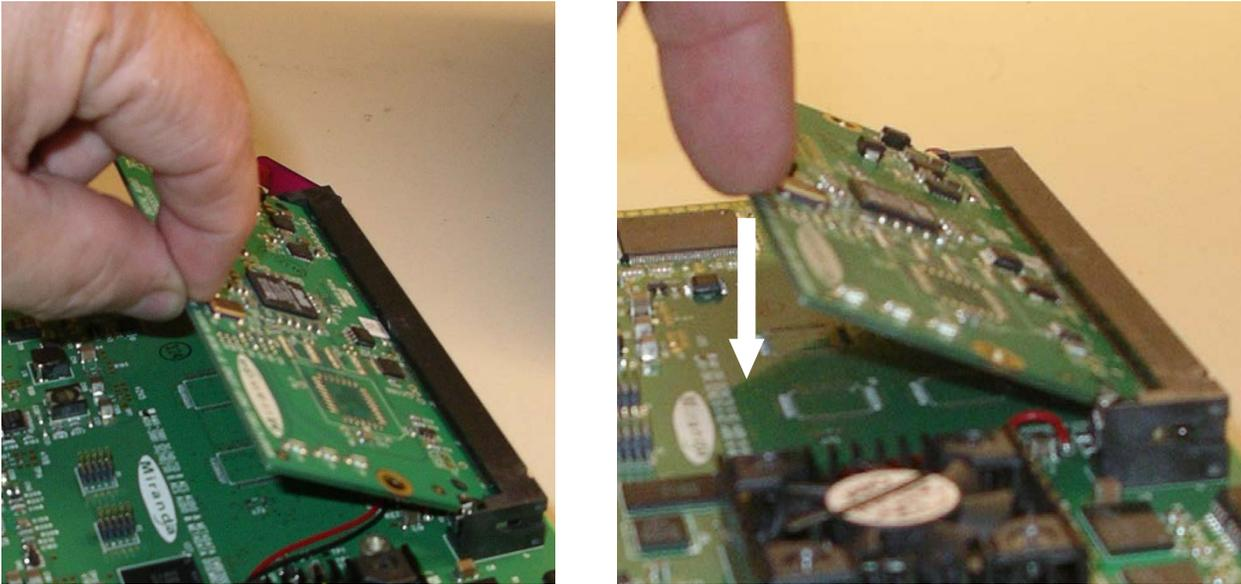
5. Push down on the module until it is parallel to the surface of the card. It will click into place
