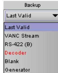
**Generator:** Use this pulldown list to turn the internal generator ON or OFF. Turning it ON selects it as the source. The generator creates a complete, specific set of metadata, which is configured in the Generator tab.
