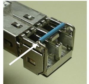
2. Position the SFP module so that the recessed slot is lined up with the tab side of the socket.
