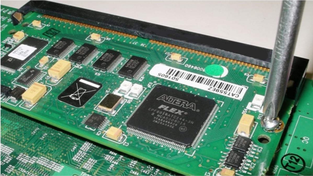
3. Push outward on the two metal clips that hold the module in the horizontal position, one located at each corner of the socket. The module will release and tilt upward
