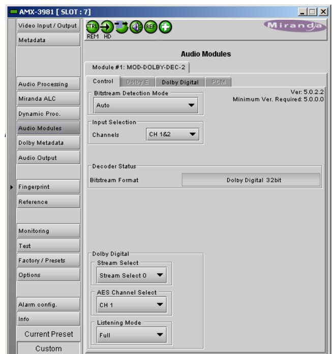
**Figure 6.1** Audio Modules - Dolby E and Dolby Digital Decoder - Control
