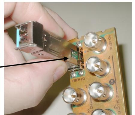
3. Slide the module straight into the socket, and push gently until it clicks into position.
