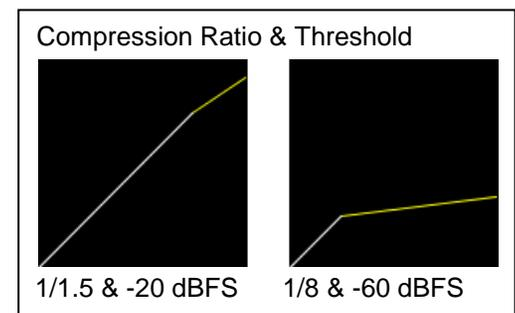
Use the *Ratio* pulldown to set the compression ratio (i.e. slope of the transfer curve). The compression ratio specifies how much the output level changes with respect to the input level:
