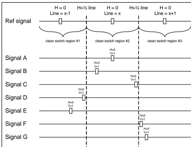
To determine whether a clean hot switch is possible, you need to determine whether the two input signals lie in the same clean switch region. There are two ways to measure the position of the signals with respect to the reference:
