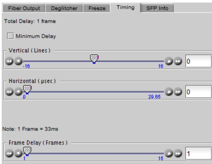
Figure 5.6 Video Input/Output – Timing tab
