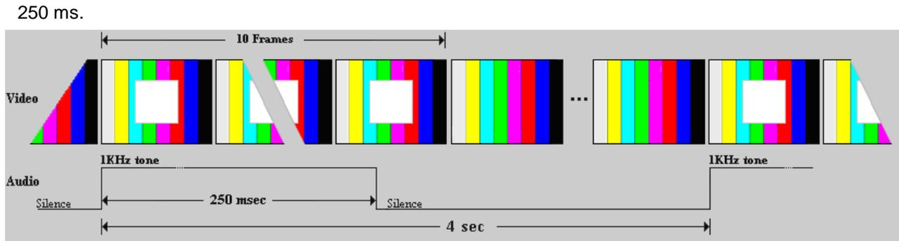
Figure 5.51 Lip Sync test signal appearance and timing
