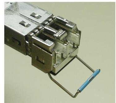
2. Grasp the SFP module between your thumb and forefinger, and pull it straight out of the slot.
