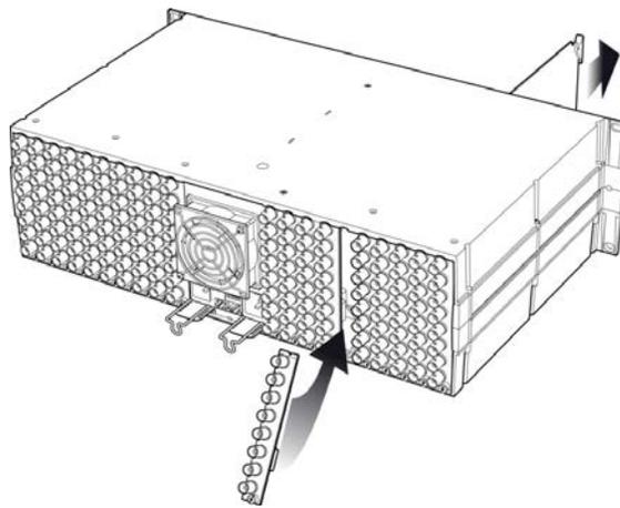
**Figure 2.1** Densité-3 frame – rear panel installation
