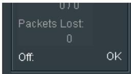
The **Off:** statistic indicates the offset of the Ancillary Stream, compared to the Video Stream. Measurement is made using Timestamp of the associated streams.
