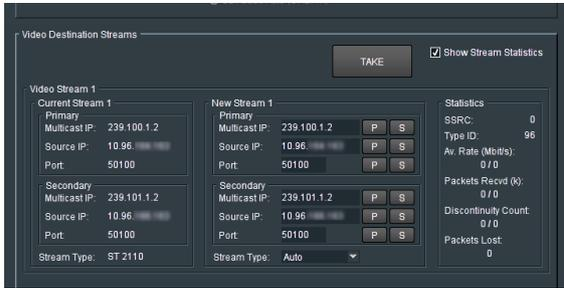
The appropriate **RTP Source** details are configured in the **Video Stream 1** menu.
