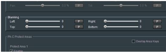
The **Blanking** slider controls allow the User to blank areas of the output image. Blanked areas will appear black in the output image.
