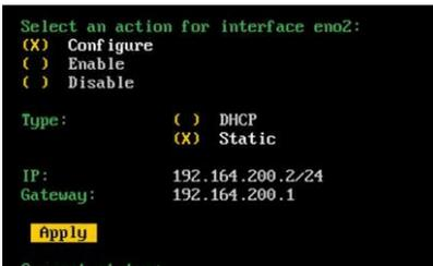
Once **IP Address** and **Gateway** have been configured, using the up/down arrows on the keyboard, navigate to and highlight: **Apply**
