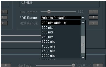
This control is only active when the conversion mode is HDR to SDR. The control is used to define the SDR brightness of the output.
