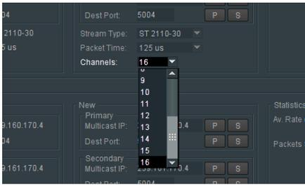
The **Channels** control allows the actual number of channels the specific stream can carry to be defined. The actual number of channels that can be configured will depend upon the **Audio Configuration** (see section 9.9.1, above).
