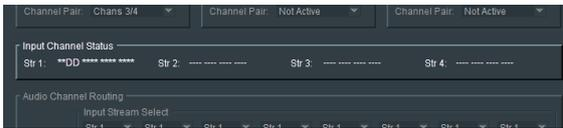
The **Input Channels Status** menu displays the actual audio present in the selected input stream.
