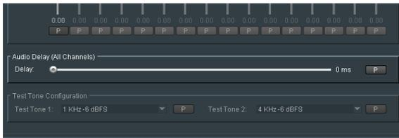
The **Delay** control allows a global delay to be applied to all audio channels. The control will delay audio relative to video.
