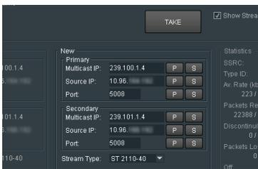
Should the input require reconfiguration to a different input, the details of the new input should be entered in the relevant **New** stream field and the **Take** button pressed to action the change.
