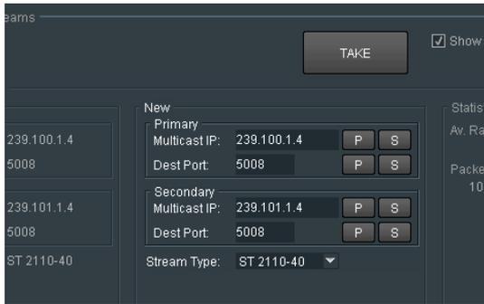
Should the input require reconfiguration to a different input, the details of the new input should be entered in the relevant **New** stream field and the **Take** button pressed to action the change.
