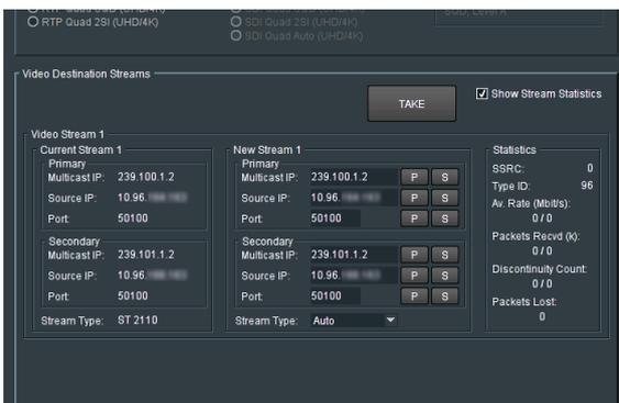
Note: The incoming RTP Streams to Alchemist Live are referred to as Destination Streams. The IP details entered will be the output side of the source device i.e. the upstream source device's destinations.
