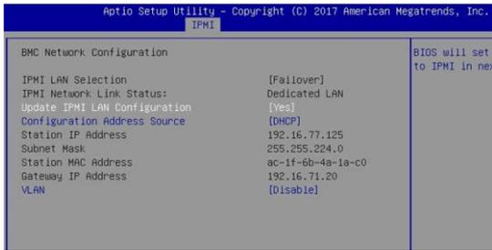
8. If it is desired to configure the address source to be a Static IP Address, select the menu item **Configuration Address Source**. A submenu will appear called **Configuration Address Source**:
