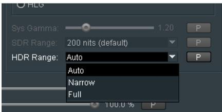
This control is only active when the output is defined to be HDR compliant. The HDR Range may be set to **Auto**, **Full** or **Narrow**, using the drop down menu.
