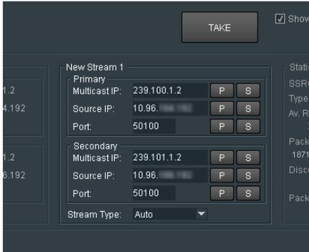
Should the input require reconfiguration to a different input, the details of the new input should be entered in each of the four **New Stream** fields and the **Take** button pressed to action the change.
