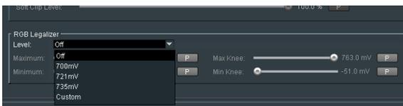
Alternatively, a **Custom** setting can be configured. When set to **Custom**, the custom controls become active allowing the User to set any combination of values:
