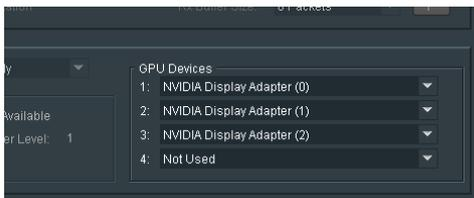
The **GPU Devices** field confirms the GPU resource available for video processing.
