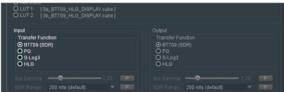
The **Input** control allows the Operator to define the input with respect to HDR.
