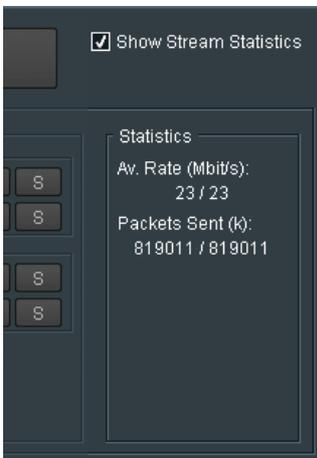
Statistics can be configured to be displayed, by checking the **Show Stream Statistics** control.
