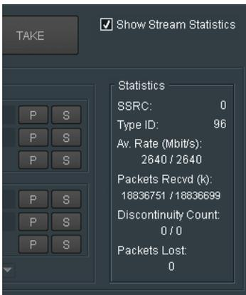
When enabled the Statistics field will detail statistics of the associated video stream. Stream statistics can be shown, or hidden, by setting the check-box **Show Stream Statistics**.
