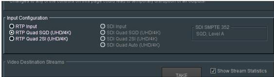
When the applied input is UHD or 4K Quad Link, the appropriate setting is either:
