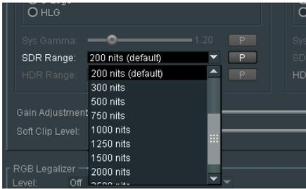
This control is only active when the conversion mode is SDR to HDR. The control is used to define how bright the SDR input is. The desired setting can be configured using the drop-down menu.
