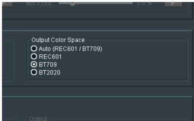
If it is desired that the output be BT2020, then the control should be set to:
