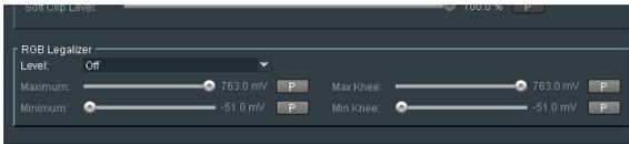
Three preset settings are offered for the RGB Legalizer **Level** control: 700mV, 721mV or 735mV. These can be selected using the drop-down menu.
