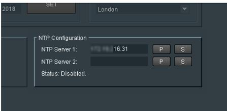
Here the NTP timestamp source can be defined. The IP Address of the NTP server can be entered and set by pressing 'S'.
