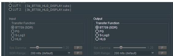
The output control allows the Operator to define the output with respect to HDR.
