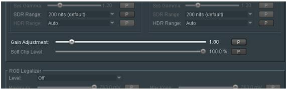
**Gain Adjustment:** this control allow the User to adjust the brightness of the output picture.
