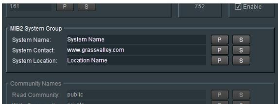
User information used to easily identify a controlled device, in this case Alchemist Live, from the SNMP control application.
