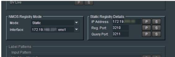
If the **Mode** is set to **Static**, the **Static Registry Details** field should be used to define the NMOS Registry.
