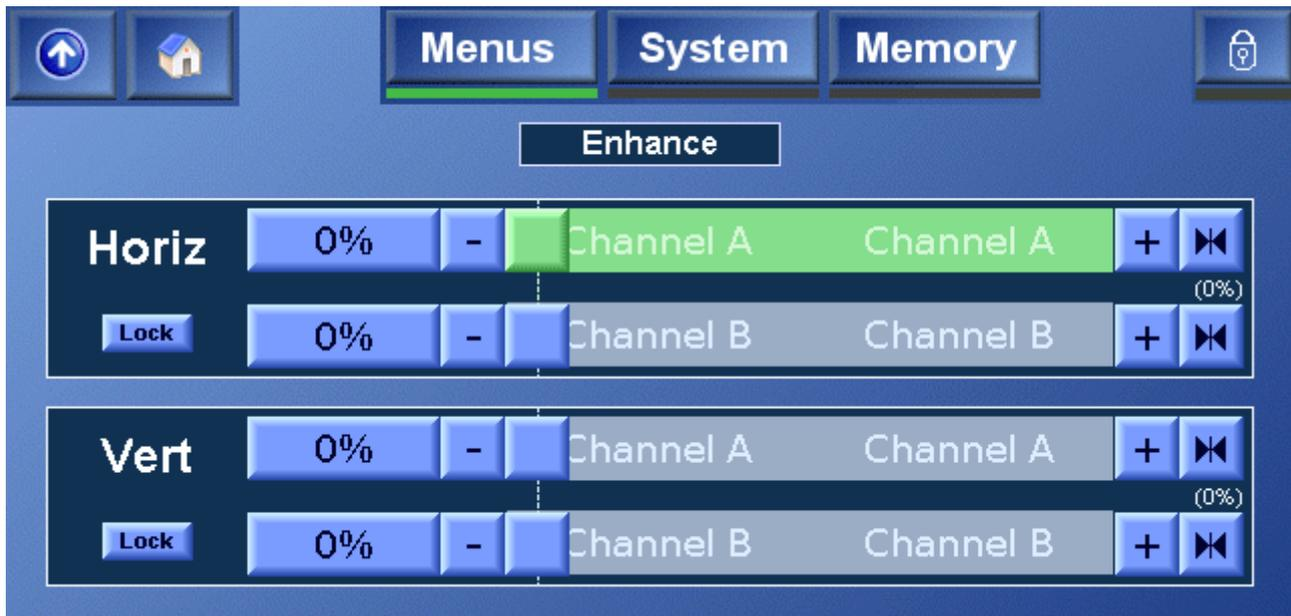
**Horiz(ontal)** This adjusts the levels of high frequency horizontal information to make the output pictures appear sharper. The enhancer range is 0 to 100% in 1% steps and the default value is 0.
