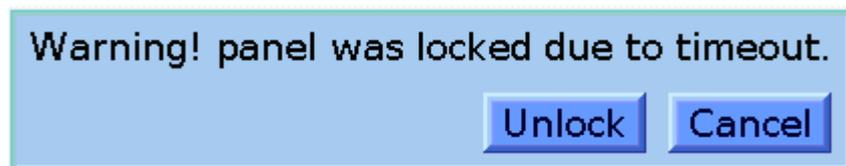
The period of time before the panel becomes locked can be set using the **Panel Timeout** control.
