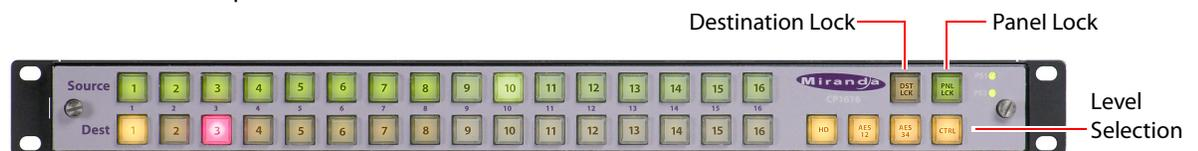
Fig. A-27: Front view of the CP1616 Control Panel
