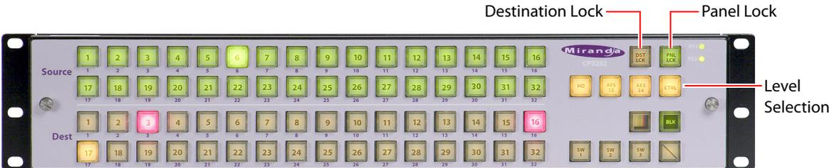
Fig. A-29: Front view of the CP3232 Control Panel
