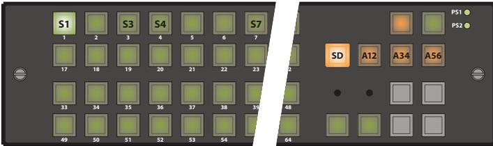
If these levels are selected, you can double-press any of the level buttons to make visible the source that contributes that level.
