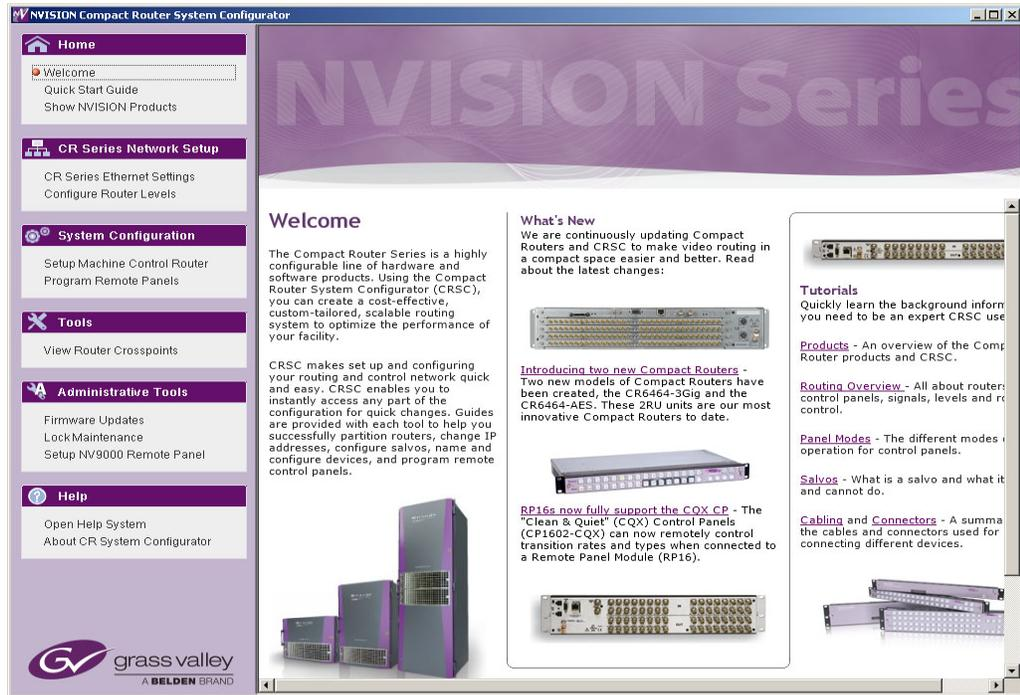
The CRSC window is divided into two main parts, a navigation pane at the left, and a work area at the right:
