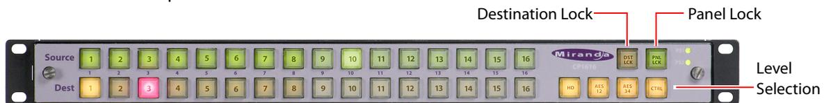
Fig. A-27: Front view of the CP1616 Control Panel
