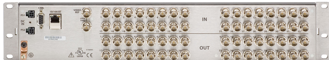
Figure 2-7. Rear View of the 32x32 3Gig, HD, SD, or AES Routers
