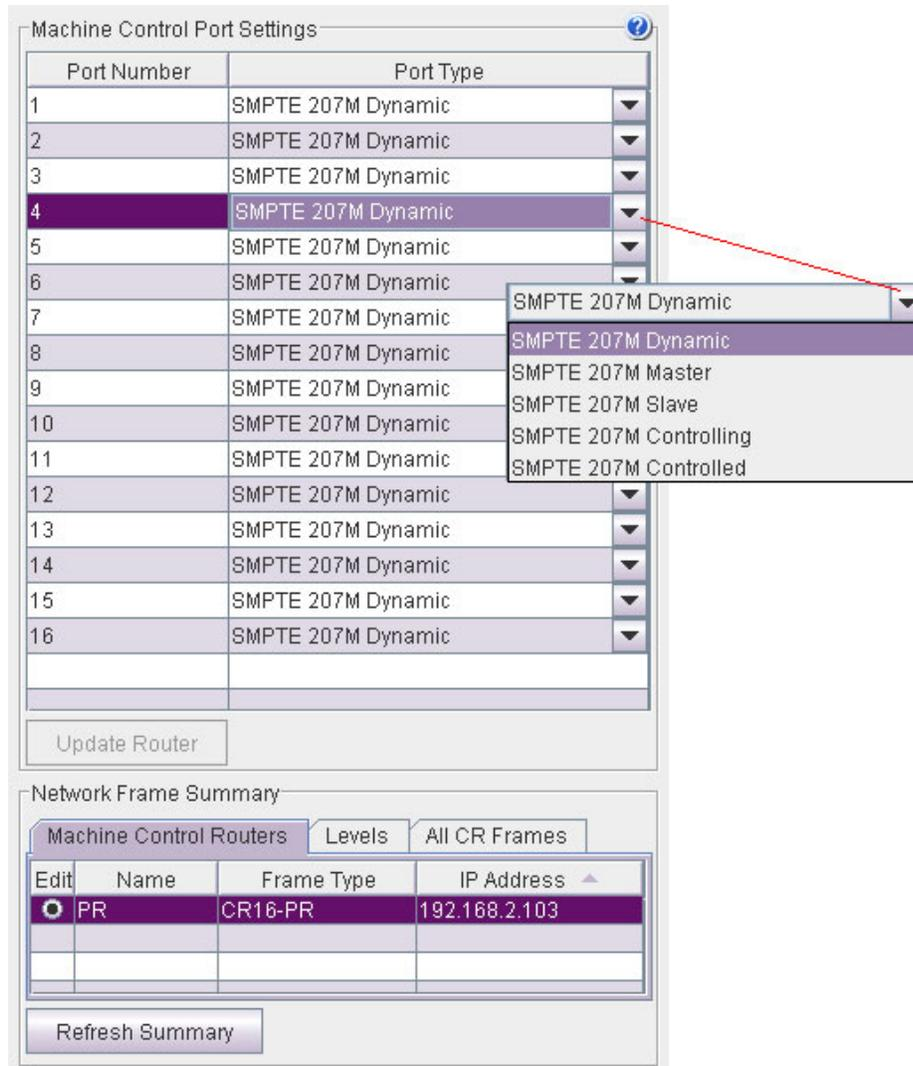
Figure 6-2. Setup Machine Control Router Page
