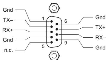
The connector is RS-485, but can be used as RS-422. Most of the compact routers allow RS-485 multi-drop now and eventually all will support it.
