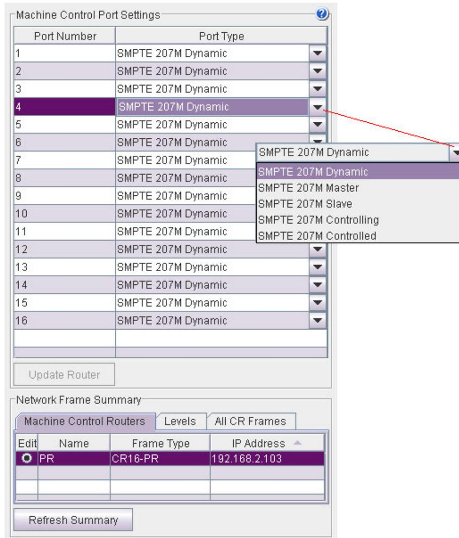
Figure 6-3. Setup Machine Control Router Page
