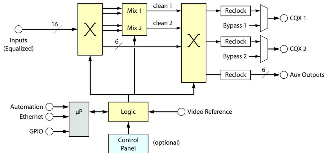
Figure 12-18. Block Diagram of the CQX Digital Video Router
