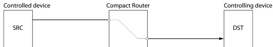
A controlling device sends commands to a controlled device. The controlled device passes responses (such as status) back to the controlling device. A source device can be a controlling device or a controlled device. A destination device can be a controlling device or a controlled device.
