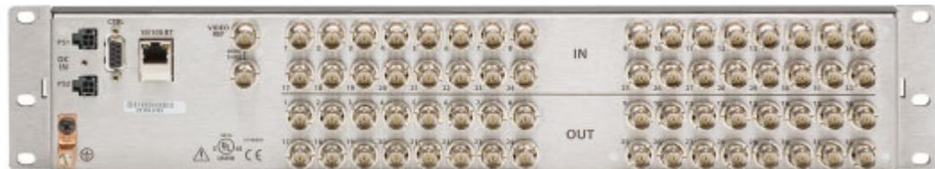
Figure 12-9. Rear View of the 32x32 3Gig, HD, SD, or AES Routers
