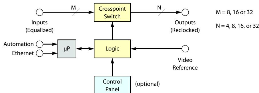
Figure 12-17. Block Diagram of the Digital Video Router
