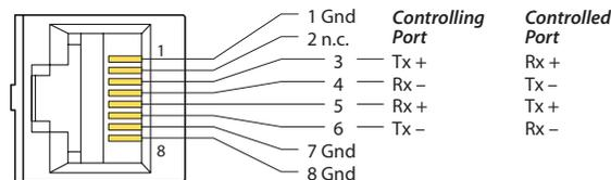
A port can be configured as “controlling” or “controlled” or variants (dynamic, master, slave). That is, the definition of the port can be reversed (Tx becomes Rx and vice versa) either during configuration or during operation.
