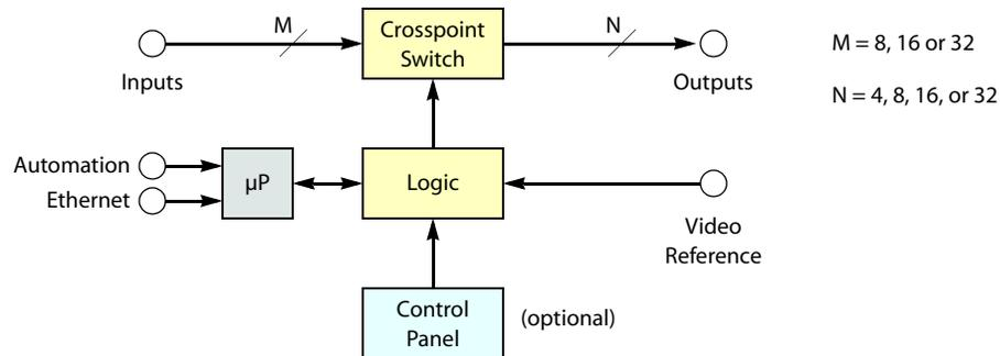
Figure 12-20. Block Diagram of the Analog Video Router
