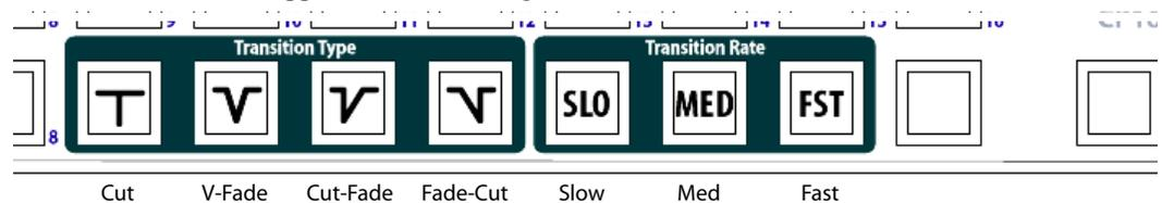
At present, a remote CQX panel’s transition rate and transition type buttons have no effect on the CQX router’s transitions. The transition rate and type buttons of a captive panel do affect transitions.
