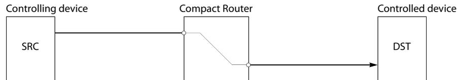
Above, the source device is a controlling device. A destination can also be the controlling device:
