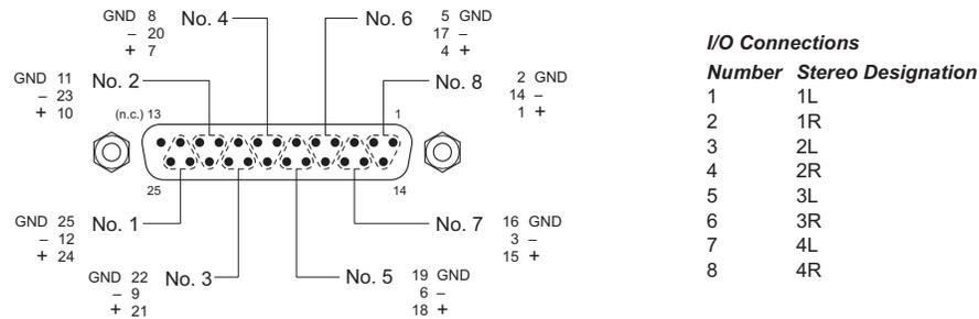
For 16×16 routers, the connectors provide inputs (or outputs) 1–8, 9–16, 17–24, and 25–32, respectively, and are labelled that way on the rear of the router. Inputs (and outputs) are treated as 16 stereo pairs.
