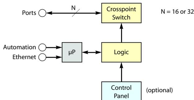
Figure 12-23. Block Diagram of the Machine Control Router
