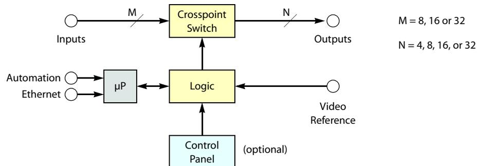
Figure 12-21. Block Diagram of the AES Router
