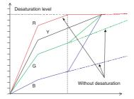
The contrast compression system used in the 1707 restores the luminance and chrominance, as well as contours in over-exposed areas, so avoiding desaturation. This enables fullest use to be made of the wide contrast range provided by the sensors and the 12-bit video processing.
