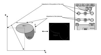
You can vary the amplitude of the contour signal as a function of colour. For example, you might reduce the amount of detail in the face to ensure satisfactory rendering of portraits.
