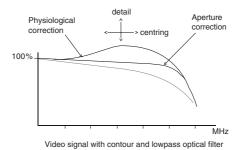
Noise suppression on the horizontal and vertical contour signals is gain controlled. The final contour correction level is reduced in the dark areas of the image to decrease noise visibility.
