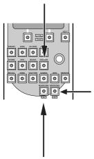
Pushing the white balance button starts the measurement. The white surface to be measured should be located in the centre of the viewfinder picture.
