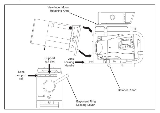
It is important that you assemble and disassemble the units in the right order. The correct order of assembly is as follows:
