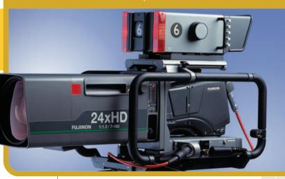
With a lightweight, ergonomic design, the LDK 6000 mk II speeds production workflows with focus-assist tools and smart cards that store image and operational settings. And its transmission system interfaces with standard triax- as well as fiber-based infrastructures for maximum flexibility.
