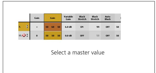
If the values are analogue they can be changed using the ROTARY CONTROLS at the bottom. If the values are select or toggle values, the selected value will be set for all camera the same.
