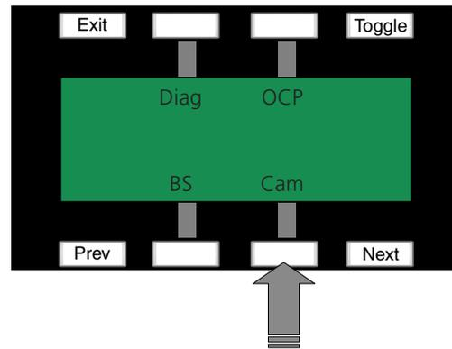
Press the selection button to choose the Camera submenu. The initial camera submenu depends on whether an SD or HD camera is connected.
