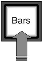
Push the **Bars** button to switch on the colour bar test signal in the connected camera. Push the button again to select a sawtooth test signal.
