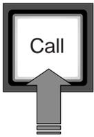
Push the **Call** button to send a signal to the connected camera calling for attention.
