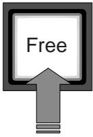
Hold down the **Free** button (10) to change the position of all the rotary controls without affecting the value of the function assigned to them. Use this button to position the Joystick without affecting the value of the iris or the master black.
