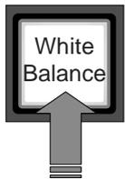
Press the **White Balance** button once to display the measurement window in the camera viewfinder.
