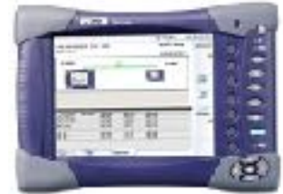
OTDR- optical time-domain reflectometer
